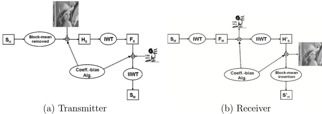
FIGURE 1. The block diagram of the proposed method. (a) Transmitter (b) Receiver
