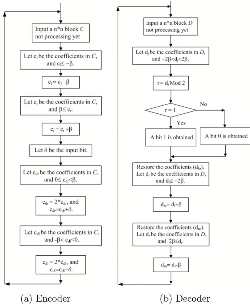
FIGURE 2. The encoder part and decoder part of the coefficient-bias algorithm. (a) Encoder and (b) Decoder.
