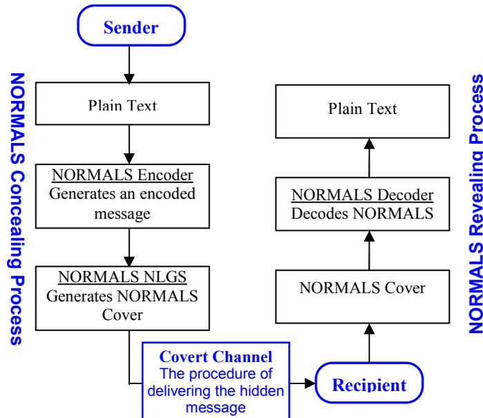
FIGURE 2. Illustrates NORMALS Communications Protocol (NCP) between sender and recipient.
