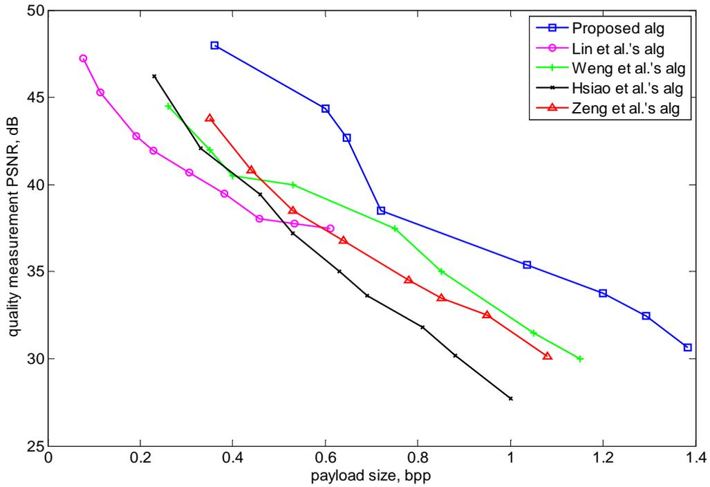
FIGURE 6. Capacity against distortion comparison on image *Lena*.
