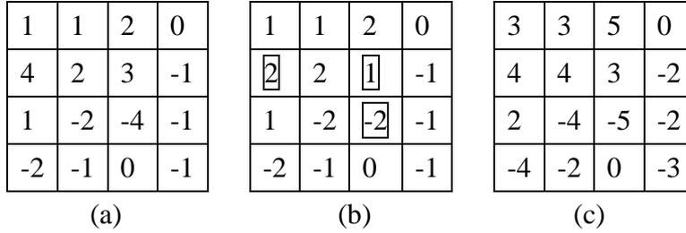
FIGURE 1. Example of 16-bit embedding with a bit-stream of 1110-0010-0010-0001. (a) The original IWT-block, (b) shifted block, and (c) bit-hidden block.
