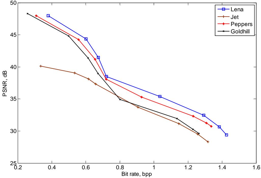
FIGURE 5. Trade-off between PSNR and bit rate for the proposed method on several images.
