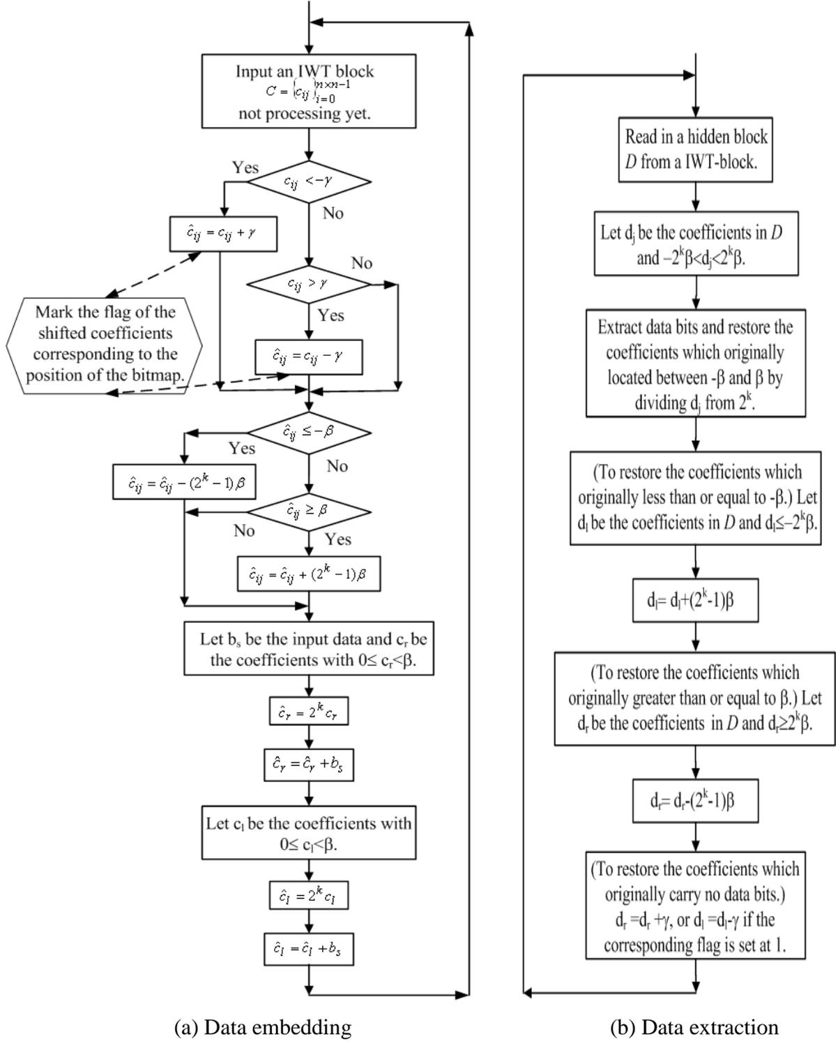
FIGURE 3. The schematic overview of the proposed method. (a) Data embedding and (b) data extraction.
