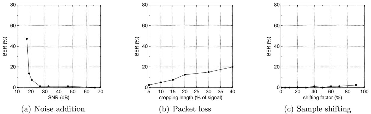
FIGURE 8. BER for spread spectrum in time domain, “natural” modifications
