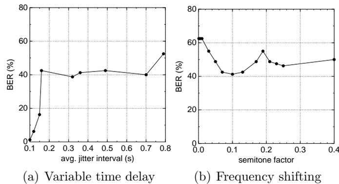
FIGURE 9. BER for spread spectrum in time domain, “malicious” modifications
