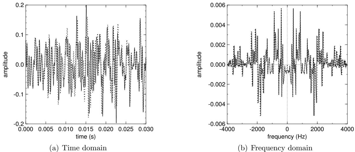
FIGURE 5. Frequency shifting, original and modified signals
