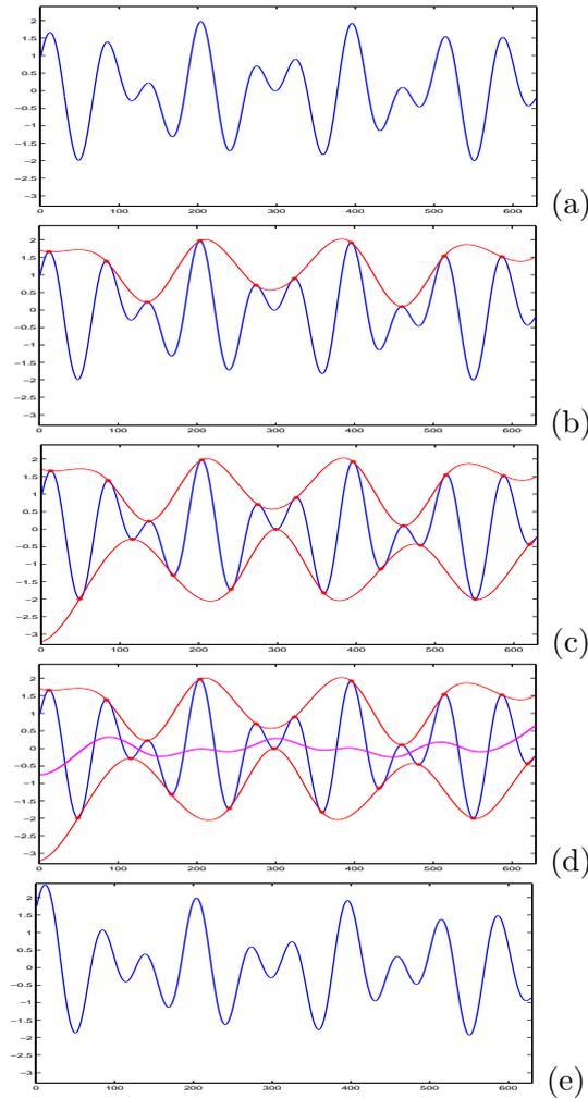
FIGURE 1. *The very first step of the sifting process. (a) is the input data, (b) identifies local maxima and plots the upper envelope, (c) identifies local minima and plots the lower envelope, (d) plots the mean of the upper and lower envelope, and (e) the residue, the difference between the input data and the mean of the envelopes.*
