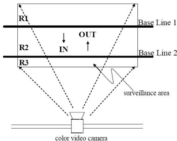
FIGURE 10. Setting of the video camera for the proposed system of vehicle flow analysis and measurement
