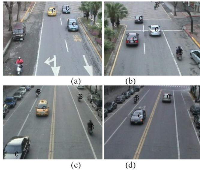
FIGURE 9. Results of vehicle classification under different traffic situations: (a) unidirectional flow in situation-1, (b) unidirectional flow in situation-2, (c) bidirectional flow in situation-1, and (d) bidirectional flow in situation-2. (Symbols C and B represent cars and bikes, respectively.)
