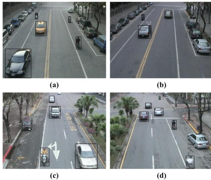
FIGURE 3. Resulting segmentation of cars and bikes under different traffic situations
