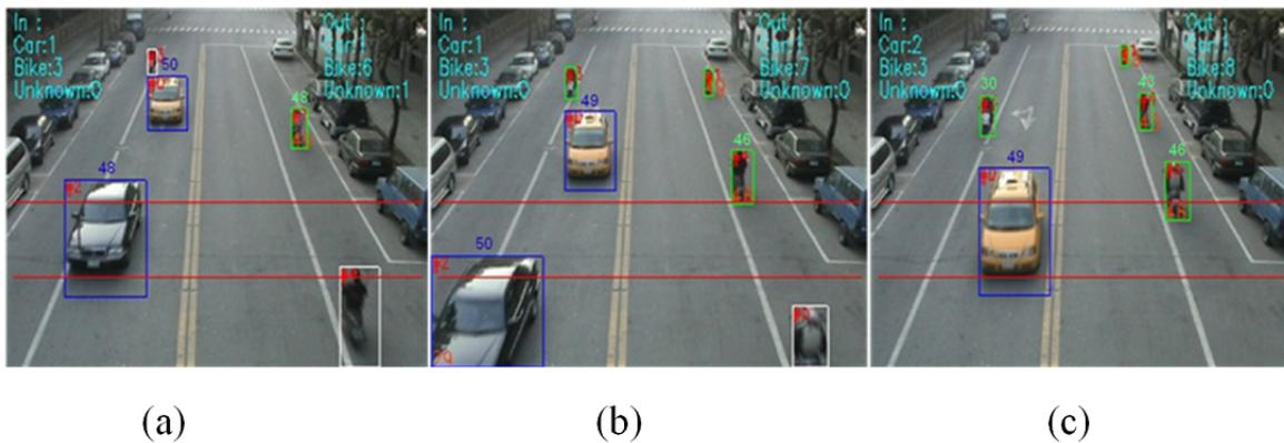
FIGURE 11. The results of the proposed vehicle flow analysis algorithm in the bi-directional two-lane way at: (a) 1575-th frame; (b) 1600-th frame; (c) 1625-th frame.
