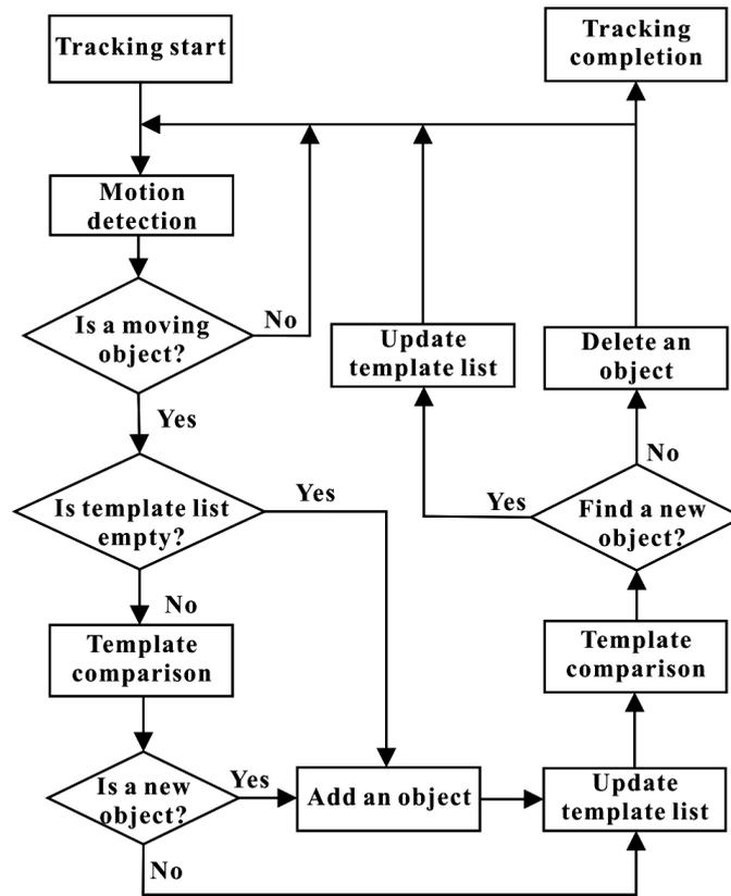
FIGURE 6. Flowchart of the proposed method for vehicle tracking
