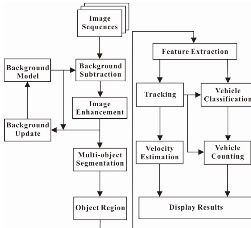
FIGURE 1. Flowchart of the proposed method for vehicle flow analysis and measurement
