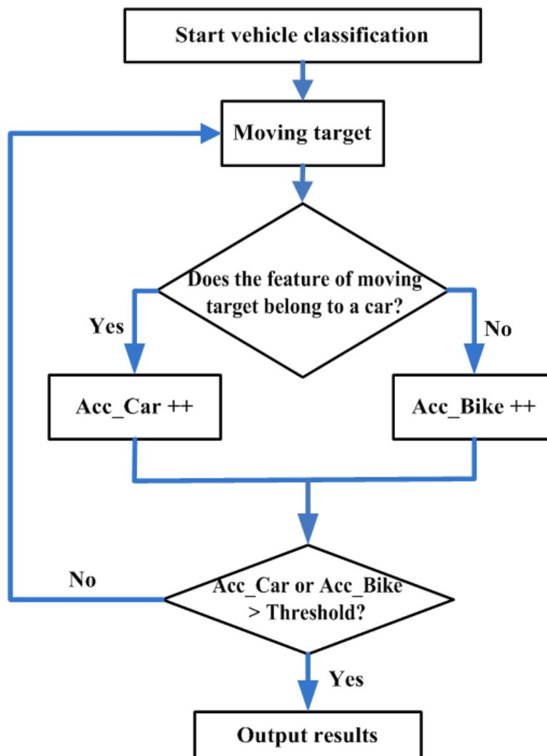
FIGURE 8. Flowchart of the proposed method for vehicle classification
