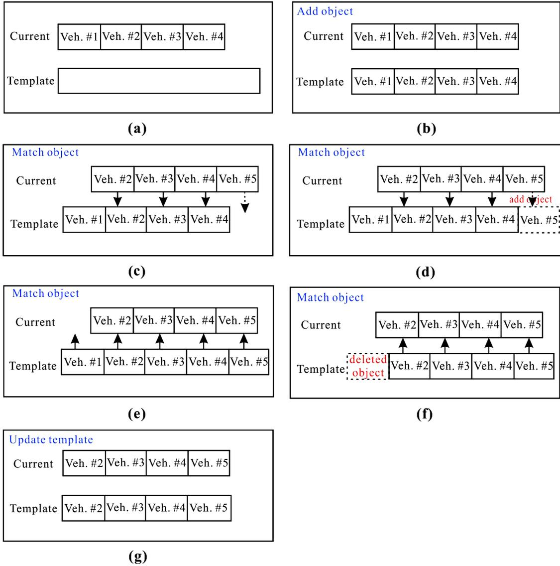
FIGURE 5. Illustration of the principle of the proposed vehicle tracking algorithm
