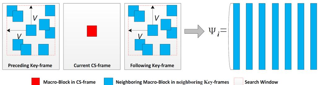
FIGURE 4. The generation of adaptive sparse dictionary for a block  $i$  in a CS-frame, it assumes that the block can be predicted using a linear combination of (vectorized) neighboring blocks in preceding and following key-frames.
