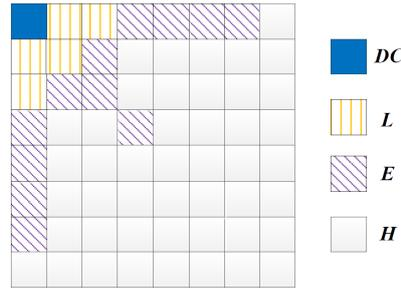
FIGURE 3. Block classification employed in our work: four indicative areas (with different marks) are fixed for all blocks.
