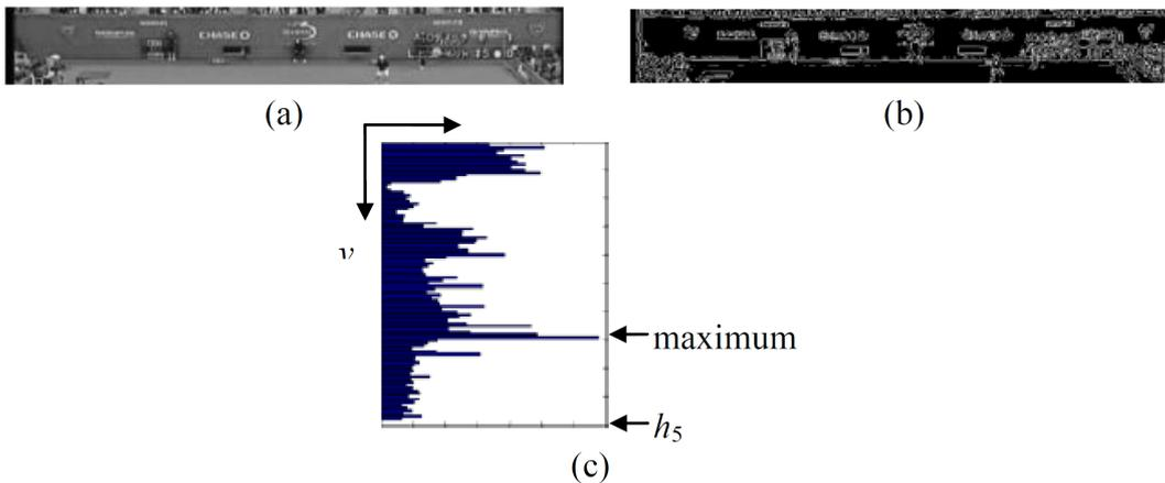
FIGURE 10. Detection of the upper bound of foutside: (A) Original image, (B) Gradient image of (A), and (C) Horizontal projection “horproj(.)” of (B).
