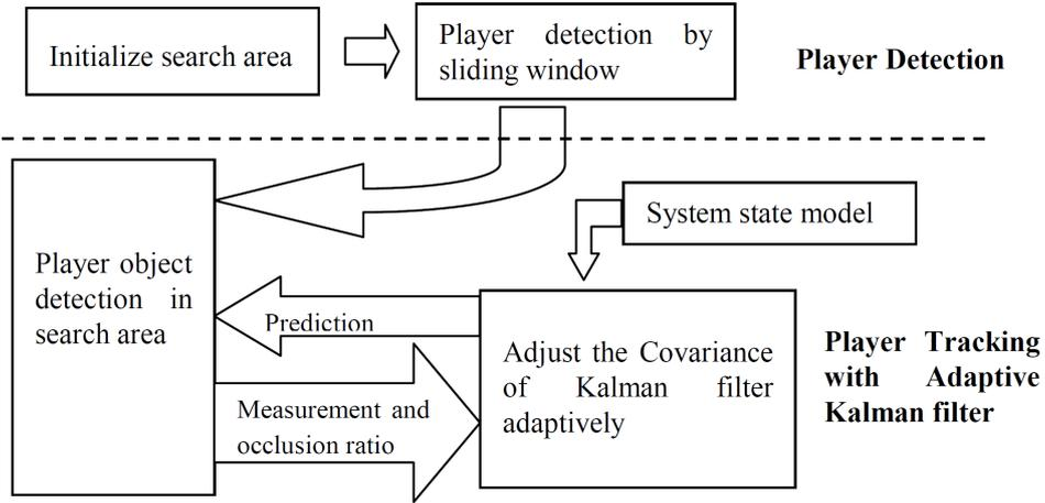
FIGURE 17. Flow chart of player tracking with adaptive kalman filter method.
