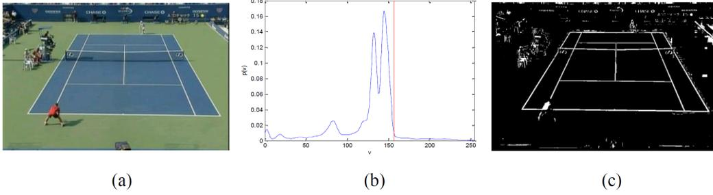
FIGURE 6. Thresholding and binarization of court lines: (A) Original image of court view, (B) Threshold determination, (C) The binarization result.
