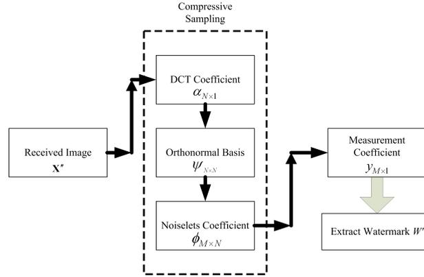
FIGURE 2. Watermark extraction with compressed sensing.
