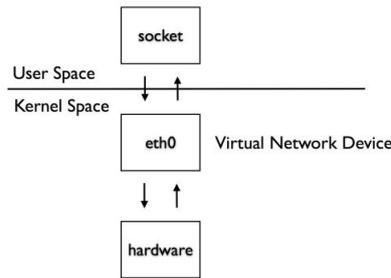
FIGURE 9. Virtual network device
