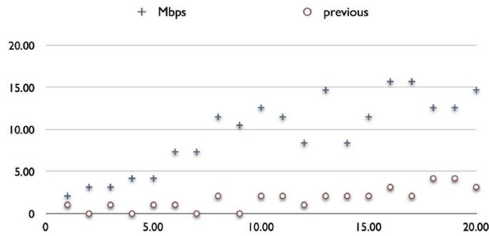
FIGURE 14. Data rate of TX with delay padding mechanism (X axis: seconds, Y axis: Mbps)
