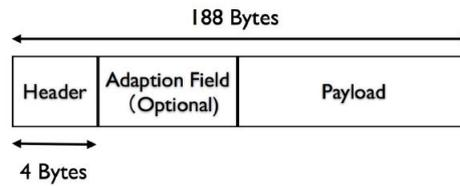
FIGURE 3. The packet format of the transport stream protocol
