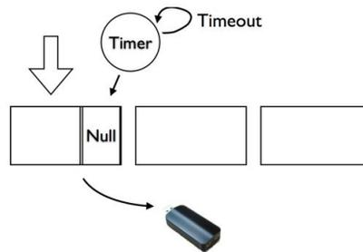
FIGURE 11. The *fast transmission mechanism* of send buffer on TX
