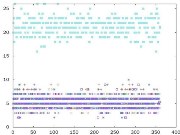
FIGURE 20. Throughput of four TCP connections (X axis: seconds, Y axis: Mb/s)
