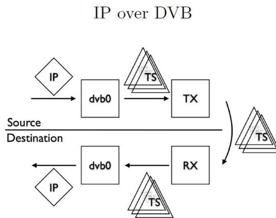
FIGURE 4. The procedure of the digital signal broadcasting
