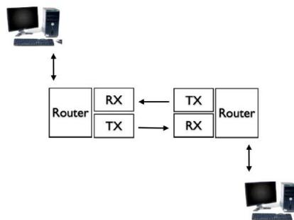
FIGURE 8. IP network backbone using wireless DVB channels
