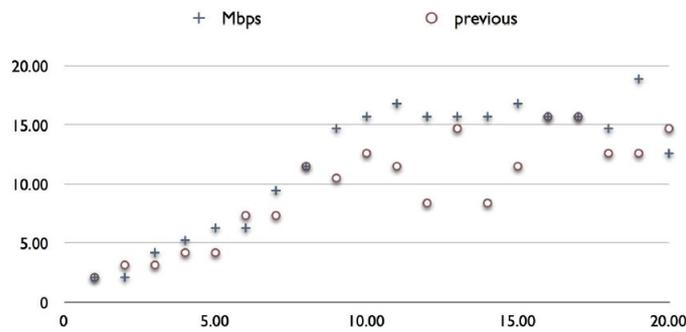
FIGURE 15. Data rate of polling mechanism with idle checking on RX ring buffer (X axis: seconds, Y axis: Mbps)
