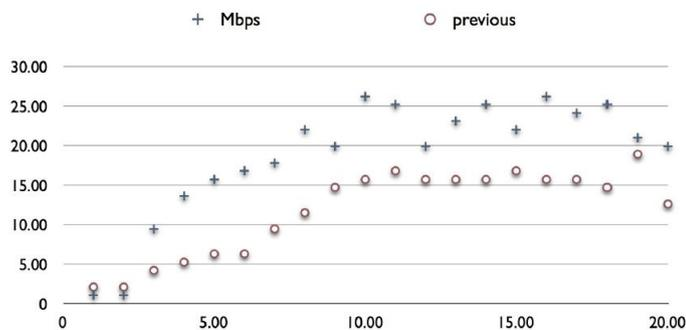
FIGURE 16. TCP throughput over DVB network (X axis: seconds, Y axis: TCP throughput in Mbps)
