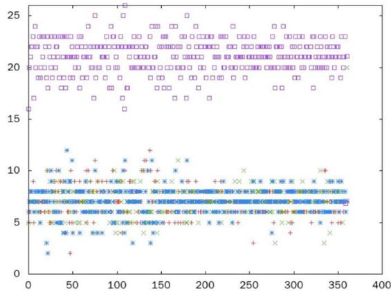
FIGURE 19. Throughput of three TCP connections (X axis: seconds, Y axis: Mb/s)
