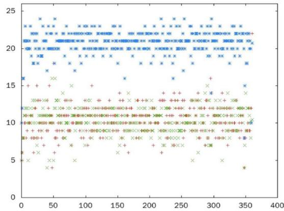
FIGURE 18. Throughput of two TCP connections (X axis: seconds, Y axis: Mb/s)
