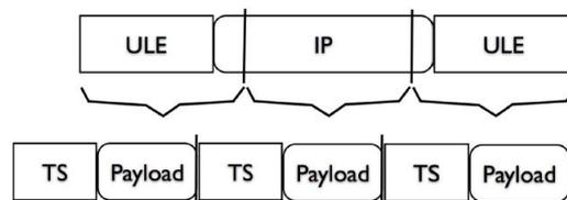
FIGURE 5. ULE packet to Transport Stream packet
