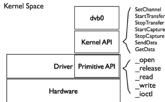
FIGURE 10. Modified architecture of driver
