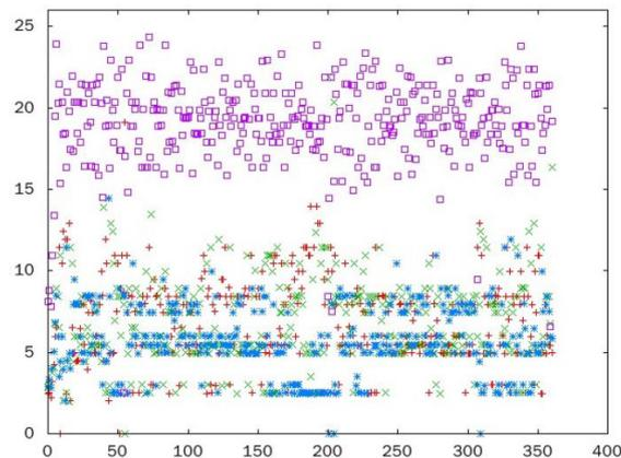
FIGURE 22. Throughput of three TCP connections (X axis: seconds, Y axis: Mbps).
