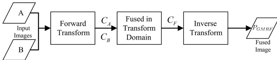
FIGURE 3. General Multi Resolution Framework (GMRF) for image fusion
