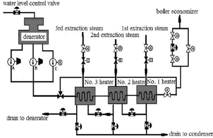
FIGURE 2. High-pressure heater system of a 600-MW unit
