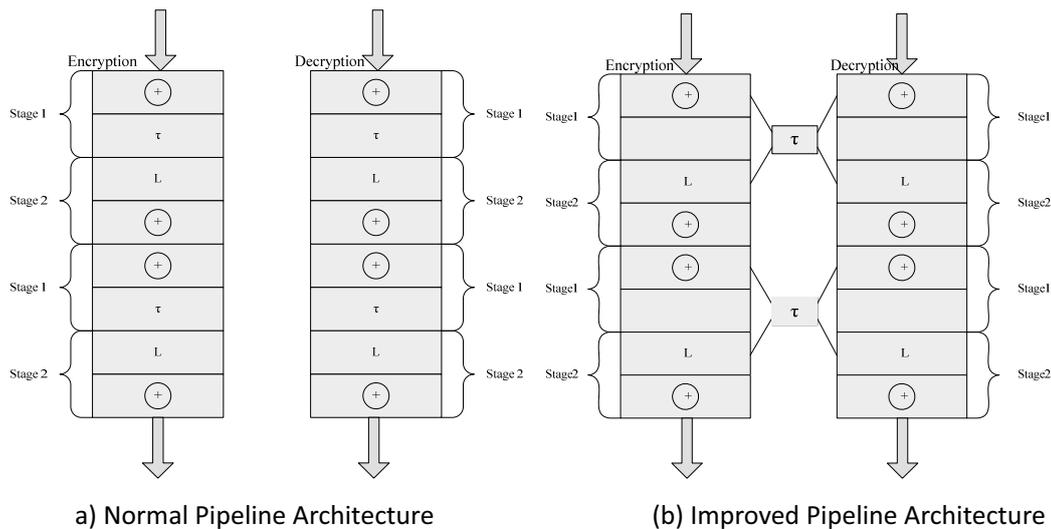
FIGURE 9. Pipeline of SM4 Algorithm
