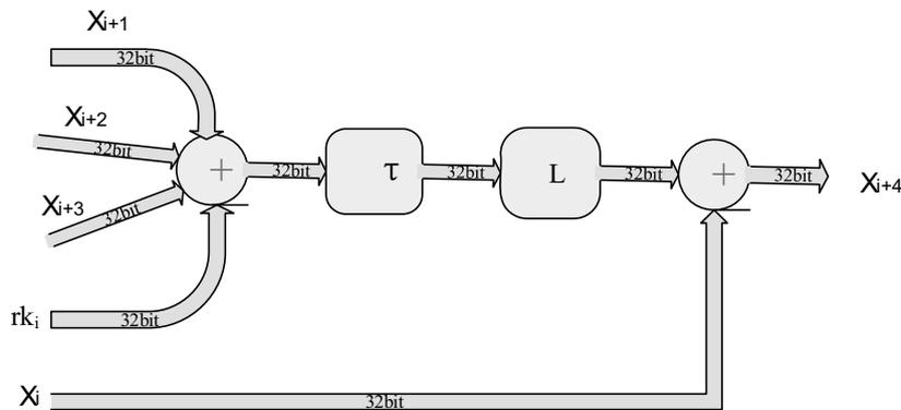
FIGURE 4. the Generation Flow of  $X_{i+4}$
