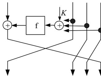
FIGURE 3. the Feistel Structure of SM4
