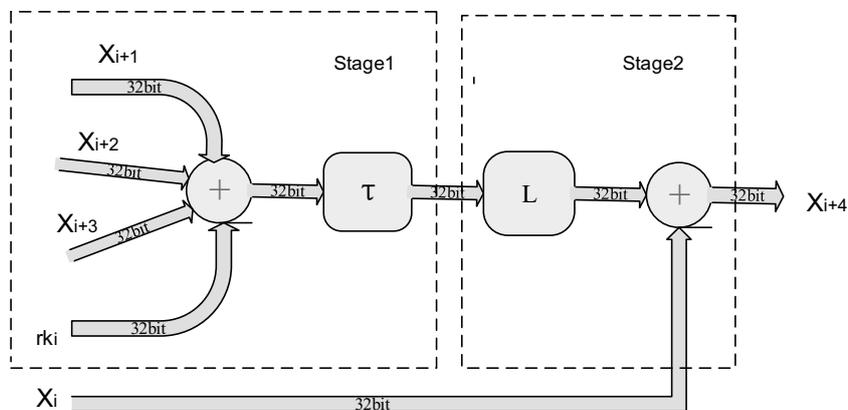
FIGURE 5. the Improvement Generation Flow of  $X_{i+4}$
