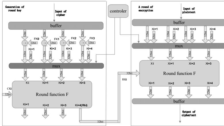
FIGURE 2. One Circle Encryption and Decryption of SM4
