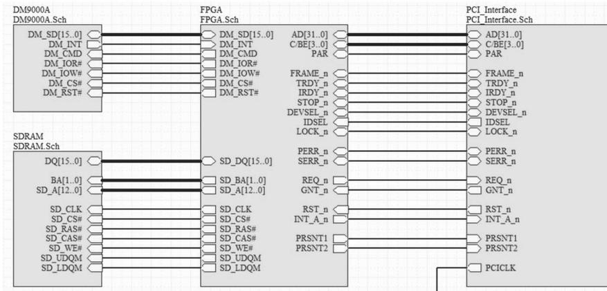
FIGURE 7. Architecture of Network Interface Card
