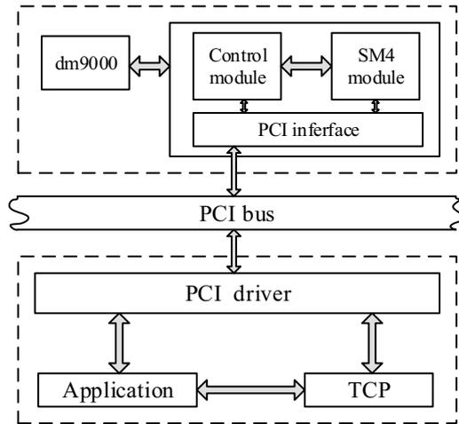
FIGURE 6. Architecture of SM4 Encryption System
