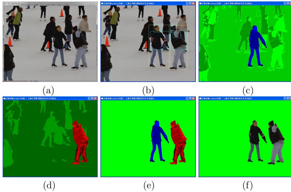
FIGURE 7. Input and experimental results of a key frame. (a) is frame 0 of standard test sequence ICE 704×576 60 orig 02 yuv. (b) shows the user input of 3 levels, 10 layers. (c) and (d) show the SCGMMs of object 1 and object 2 at level 1. (e) and (f) are the results in mask of the SCGMMs image and the original frame.
