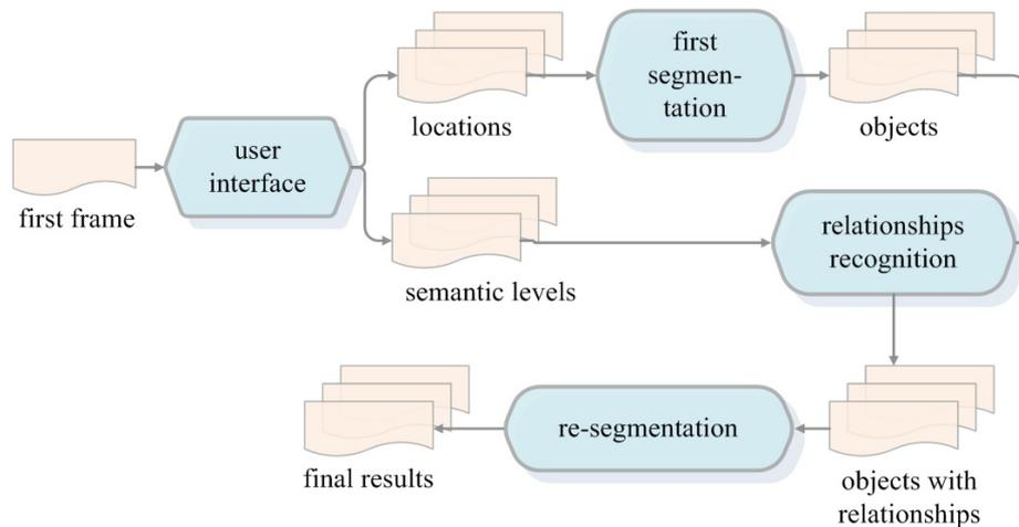
FIGURE 3. Framework of our twice-segmentation algorithm for the key frame of a video sequence
