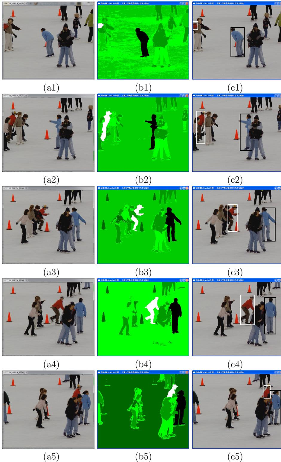
FIGURE 9. Segmentation and tracking results of subsequent frames. (a1)~(a5) in the first column: frame 200, 244, 299, 321 and 343 of standard test sequence ICE 704  $\times$  576 60 orig 02 yuv respective. (b1)~(b5) in the second column: segmentation results of corresponding frames at level 1. (c1)~(c5) in the last column: tracking results of corresponding frames.
