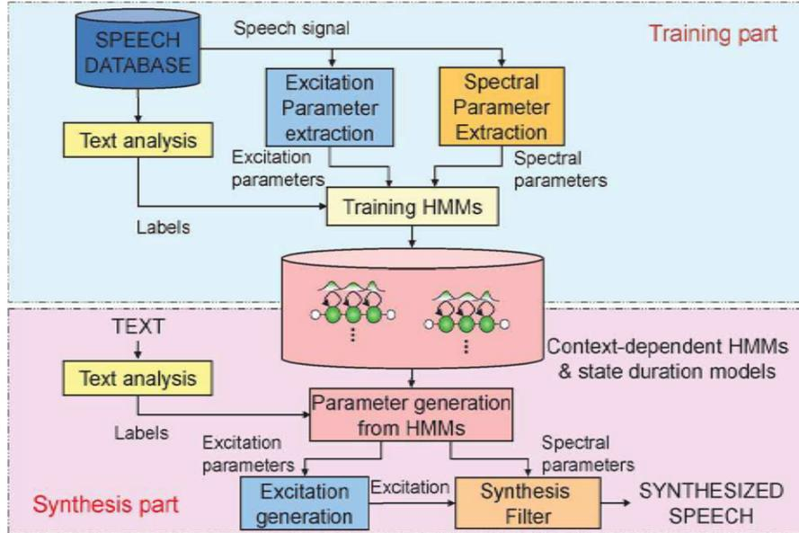
FIGURE 1. An overview of the basic HMM-based speech synthesis system [5]
