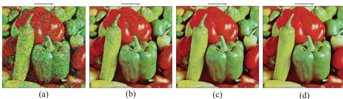
FIGURE 5. Reconstructed image of our scheme with the indicated BER and the resulting  $PSNR$ : (a)  $BER = 2 \times 10^{-2}$ ,  $PSNR = 14.68dB$ ; (b)  $BER = 3 \times 10^{-3}$ ,  $PSNR = 21.41dB$ ; (c)  $BER = 8 \times 10^{-4}$ ,  $PSNR = 26.51dB$ ; (d)  $BER = 2 \times 10^{-4}$ ,  $PSNR = 32.60dB$
