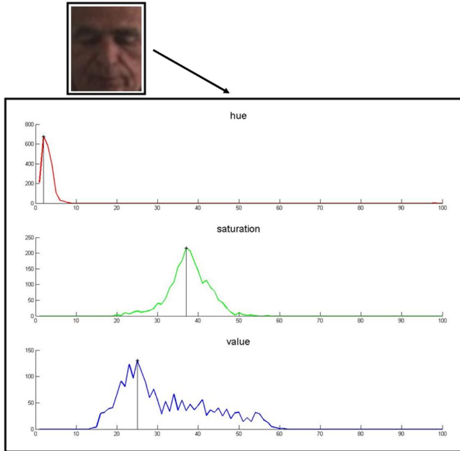
FIGURE 4. *Calculation of person-specific thresholds for skin color segmentation.*
