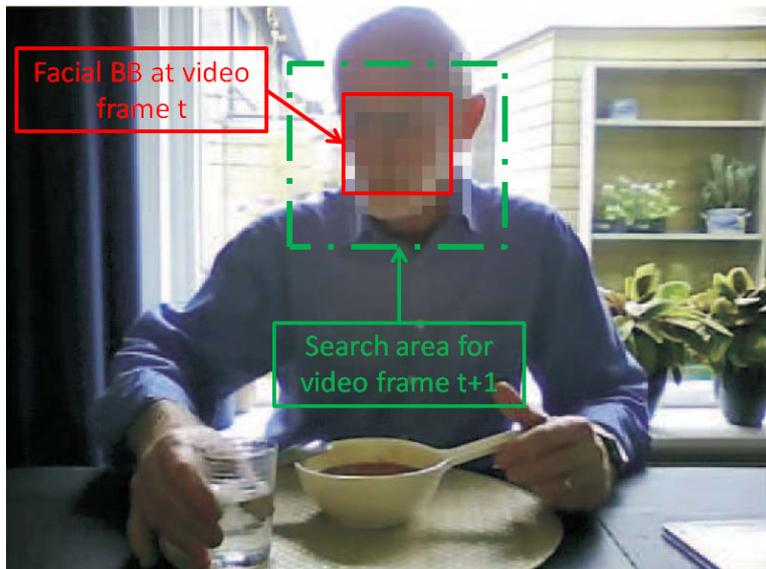
FIGURE 2. Face detection on a restricted video frame area for faster operation.
