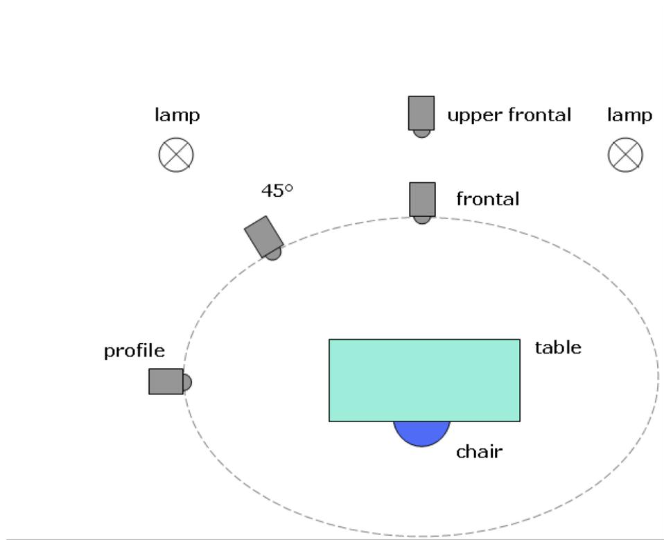
FIGURE 9. *The database camera setup.*
