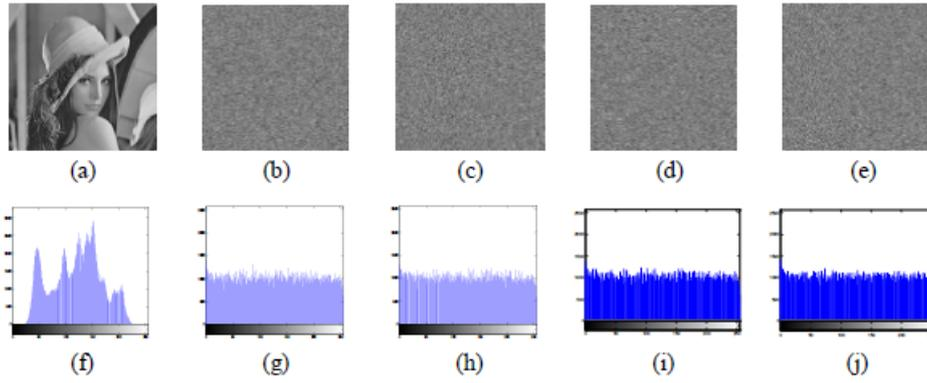
FIGURE 7. Histograms of the plain image and cipher images : (a) plain image, (b) cipher image 1, (c) cipher image 2, (d) cipher image 3, (e) cipher image 4, (f) histograms of plain image, (g) histograms of cipher image 1, (h) histograms of cipher image 2, (i) histograms of cipher image 3, and (j) histograms of cipher image 4
