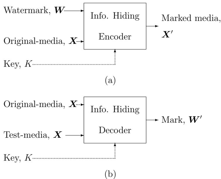
FIGURE 2. The block diagrams for information hiding [1, 2]. (a) Information insertion. (b) Information extraction.
