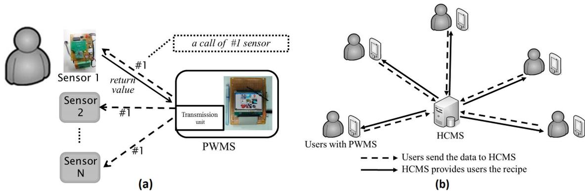
FIGURE 2. (a) Polling commands between a transmission unit and sensors; (b) A service scenario of HCMS.
