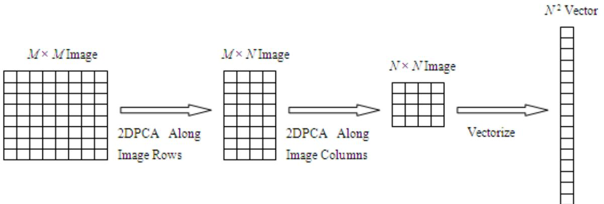
FIGURE 5. Block diagram of proposed B2DPCA
