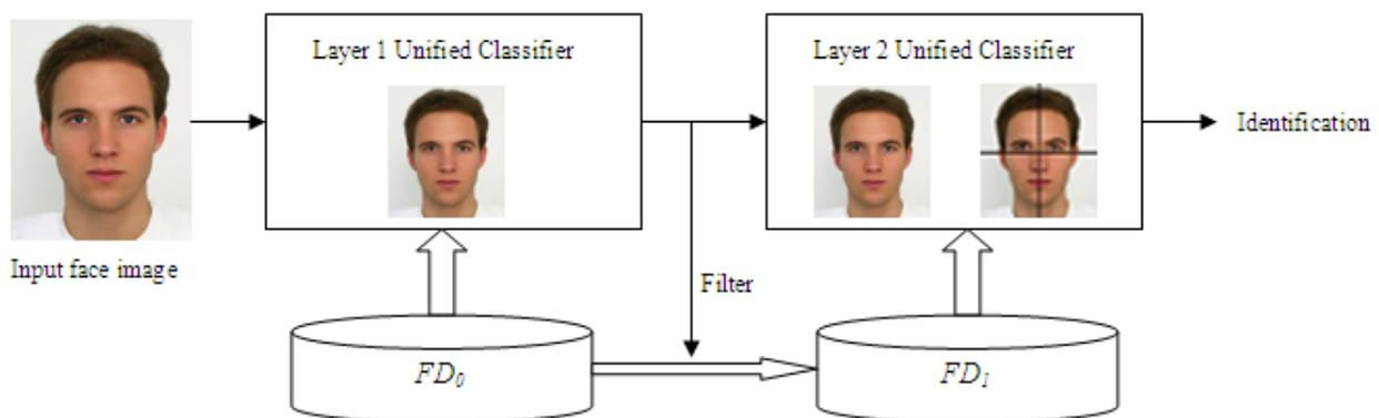
FIGURE 6. Serial integration of classifiers for face recognition
