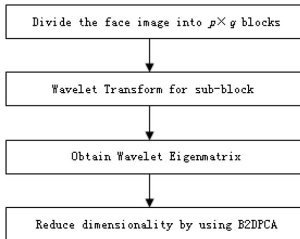
FIGURE 2. The flow diagram of blocking wavelet transforms
