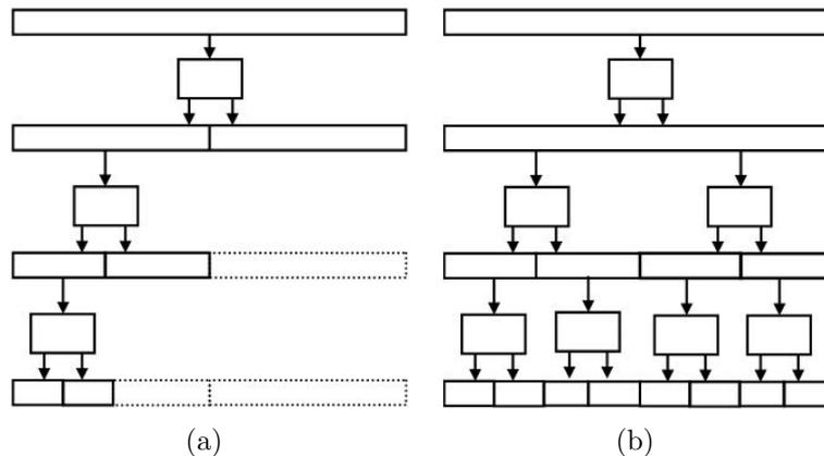
FIGURE 2. Wavelet (a) and wavelet packet (b) decomposition of one dimension signal
