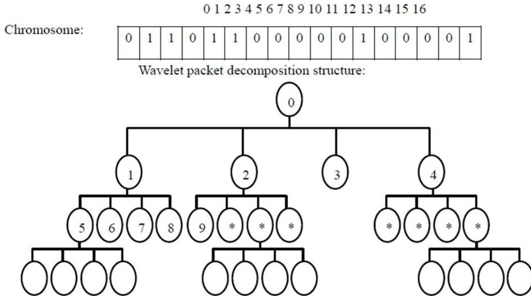
FIGURE 5. Chromosome and wavelet packet decomposition structure
