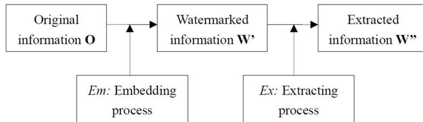
FIGURE 1. The basic framework of digital watermarking systems
