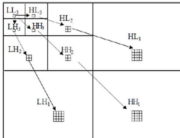
FIGURE 6. Three-level wavelet orientation tree
