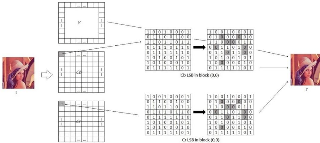
FIGURE 3. Illustration of YCbCr color space watermark embedding phase
