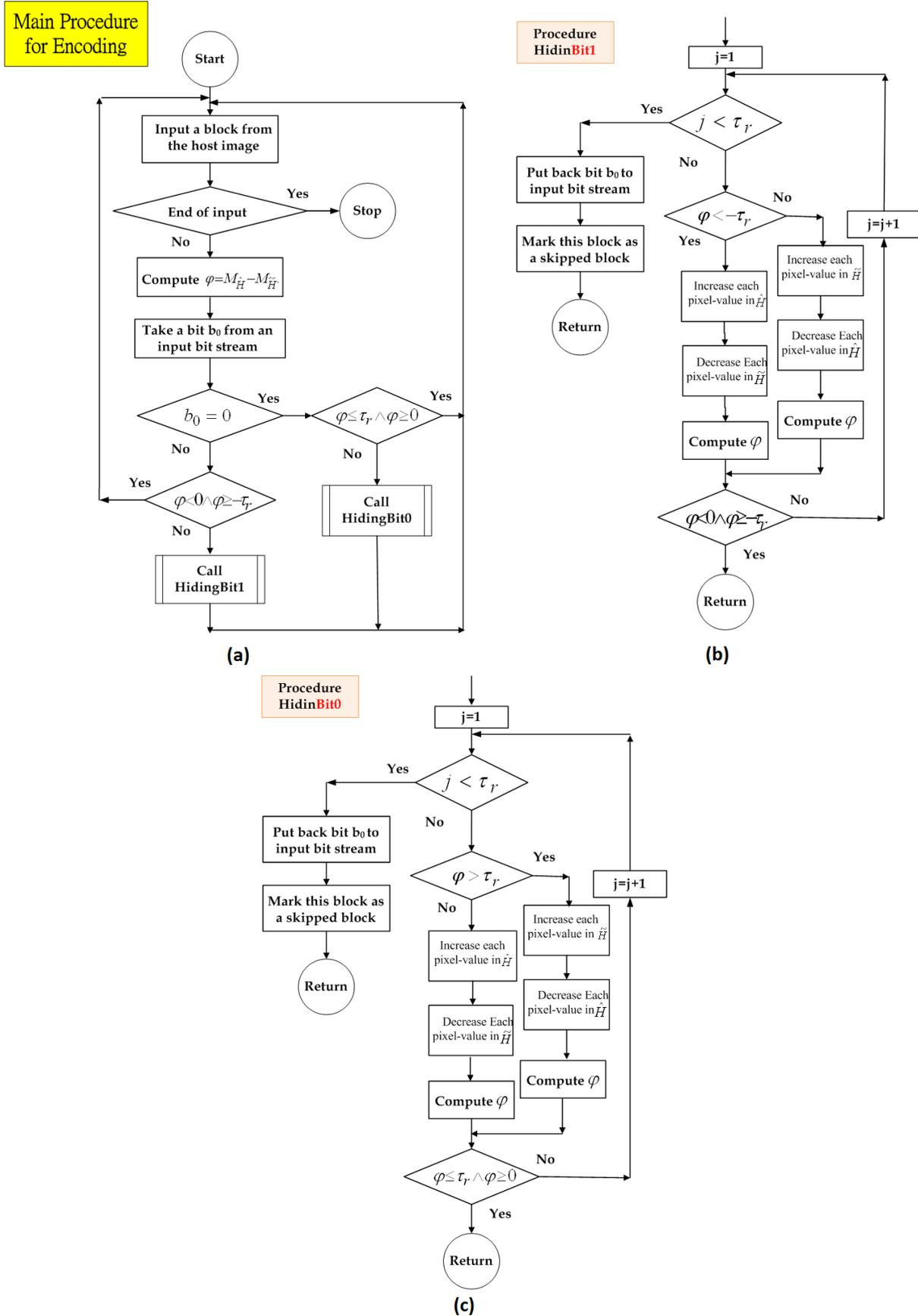
FIGURE 2. Flowcharts of our proposed bit-embedding algorithm: (a) main procedure, (b) HidingBit1 procedure, and (c) HidingBit0 procedure.
