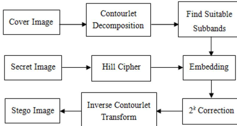
FIGURE 2. Block diagram of data embedding in contourlet domain
