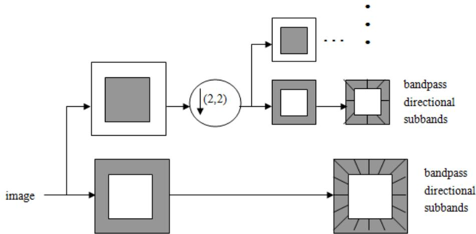
FIGURE 1. The diagram of the contourlet transform
