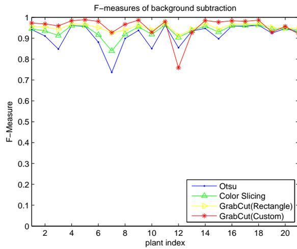
FIGURE 8. F-measures of different background subtraction methods.
