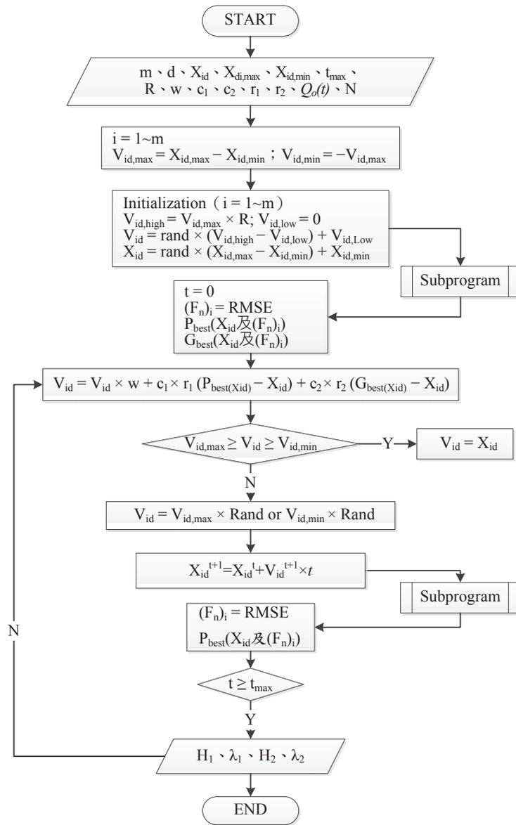
FIGURE 5. Flowchart of the main program for obtaining PTM parameters through PSO.
