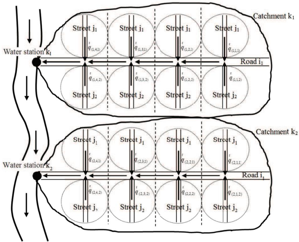
FIGURE 1. Schematic of urban-drainage grid concep.
