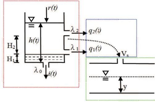
FIGURE 2. Dual model system of para-tank mechanism and sewer drainage system.
