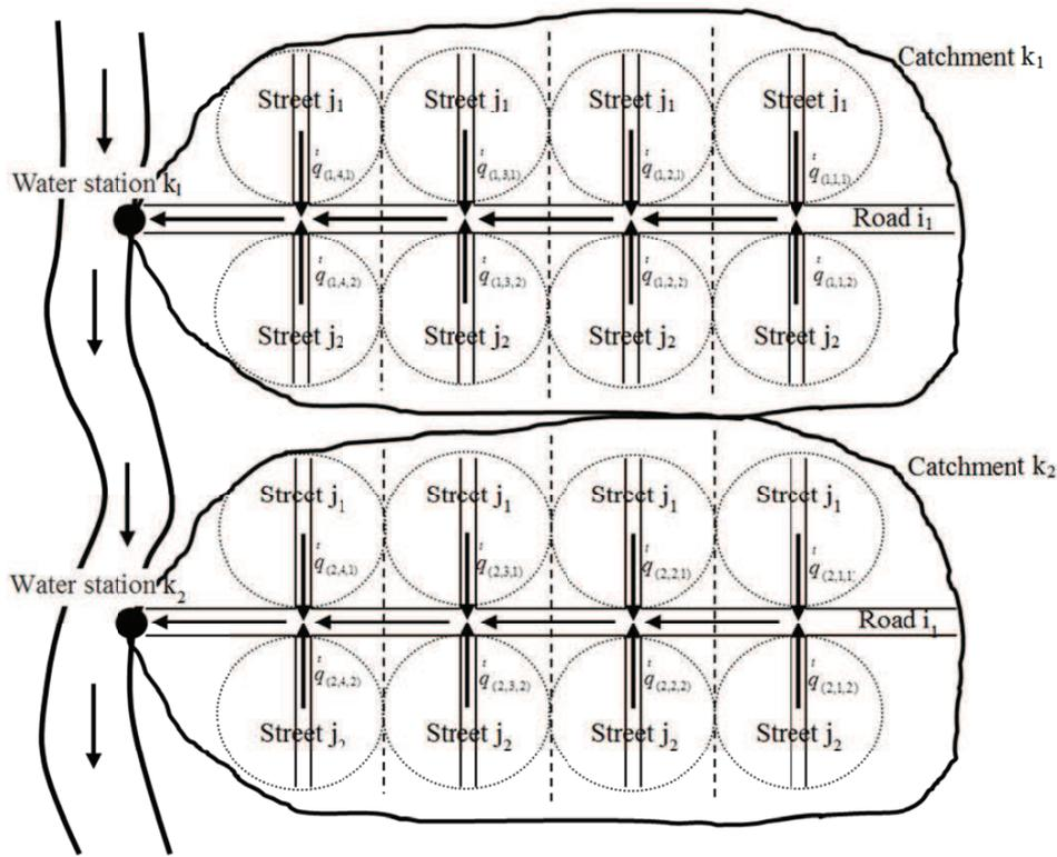
FIGURE 1. Schematic of urban-drainage grid concep.
