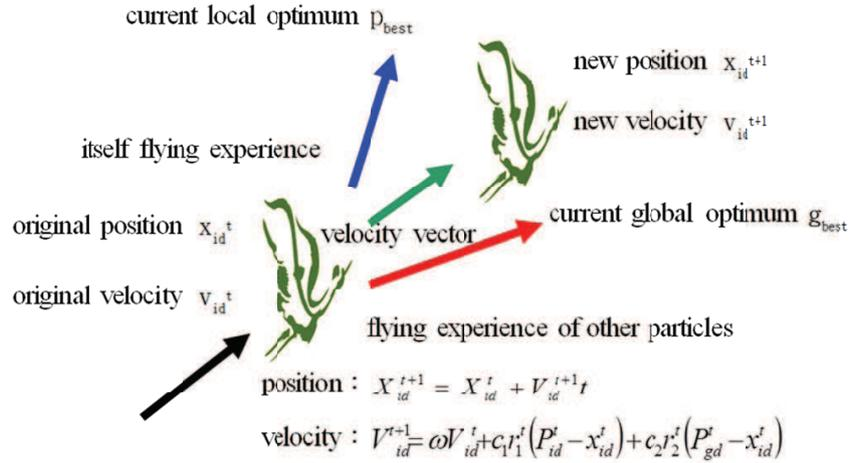
FIGURE 4. Schematic diagram of PSO.
