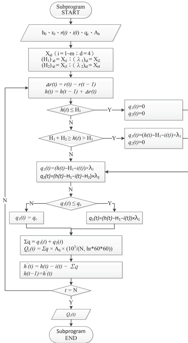
FIGURE 6. Flowchart of the subroutine for obtaining PTM parameters through PSO.
