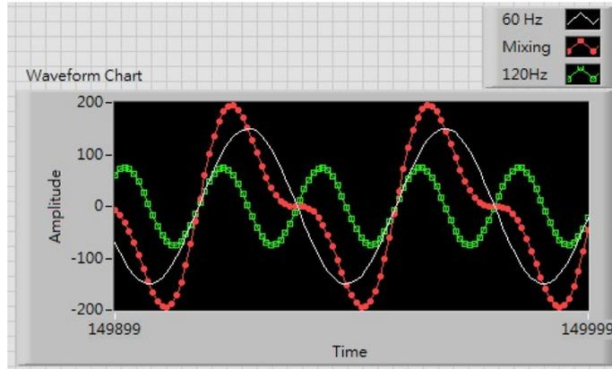
FIGURE 4. The mixed signal of the fundamental signal and its second harmonic
