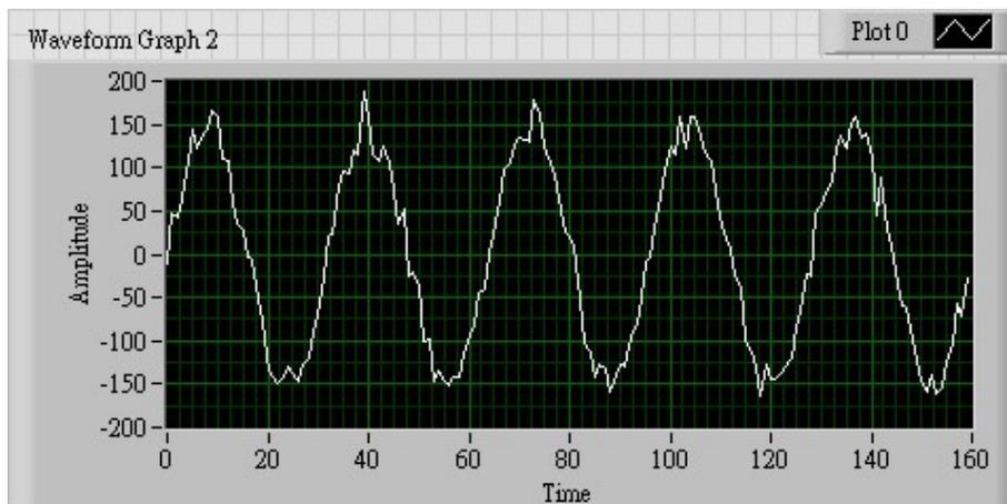
FIGURE 9. The fundamental signal with white noise
