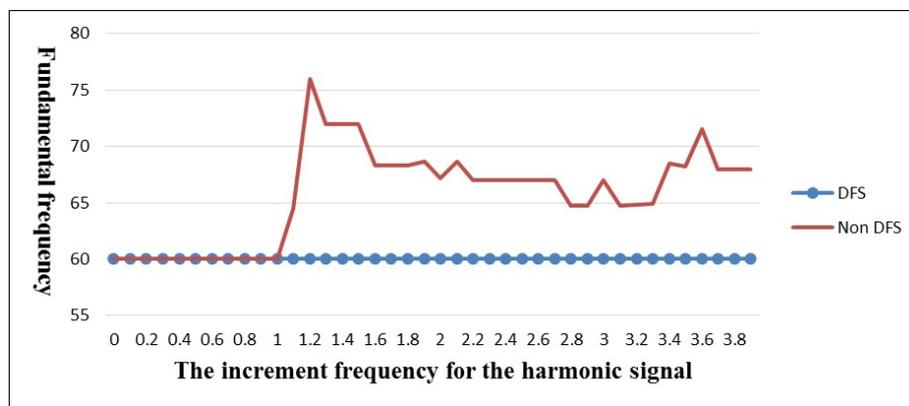
FIGURE 11. The influence of inter-harmonics on the zero-crossing algorithm
