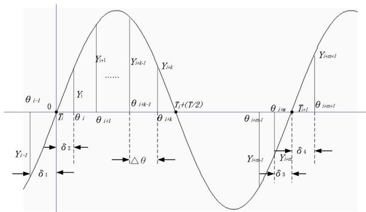
FIGURE 3. Schematic for zero crossing algorithm
