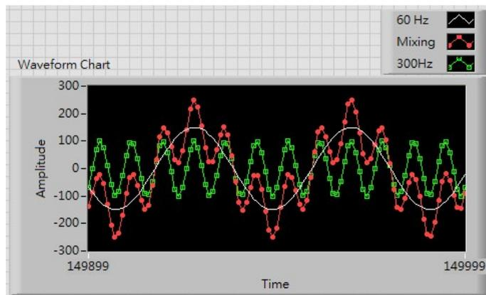
FIGURE 6. The Mixed signal of fundamental signal and its fifth harmonic
