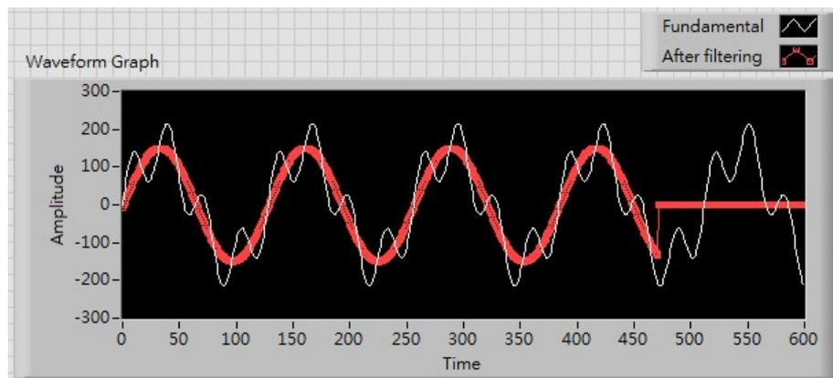
FIGURE 8. The signal with DFS implementation
