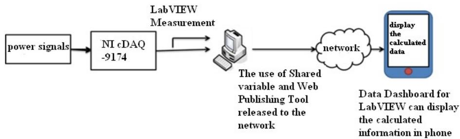
FIGURE 1. Measurement Schematic for fundamental frequency analysis of the power signal.
