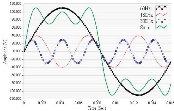
FIGURE 2. The fundamental signal with its 3rd and 5th harmonics
