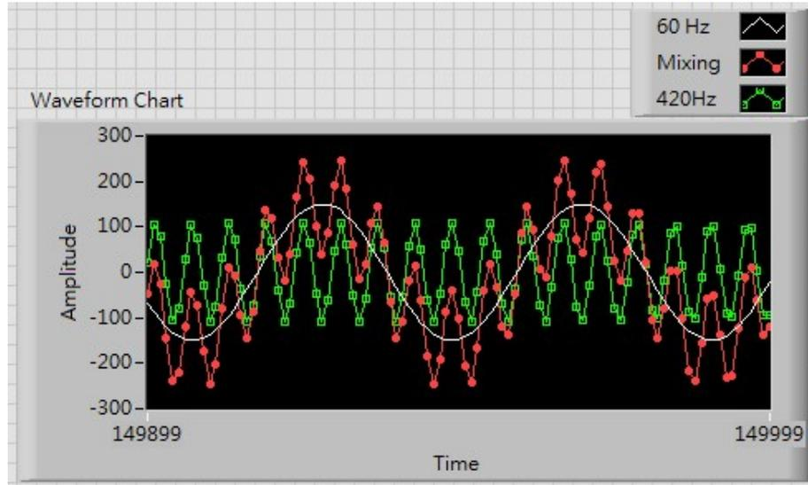
FIGURE 7. The Mixing signal of fundamental and its senenth harmonic
