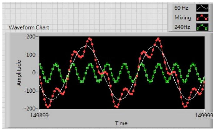
FIGURE 5. The Mixed signal of the fundamental signal and its fourth harmonic
