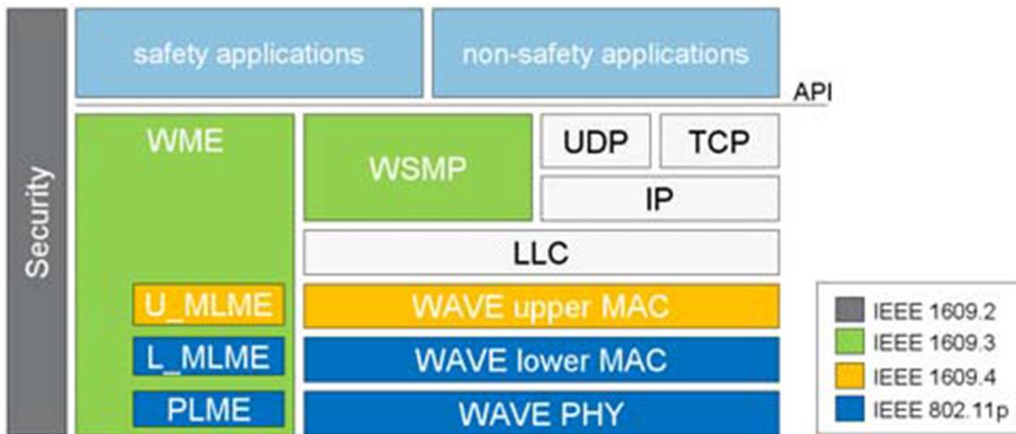
FIGURE 10. DSRC protocol architecture diagram [17]
