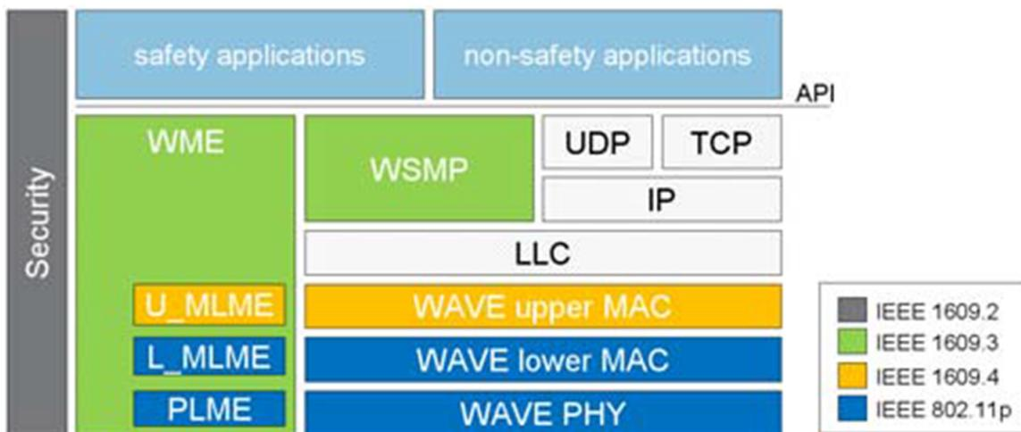
FIGURE 10. DSRC protocol architecture diagram [17]
