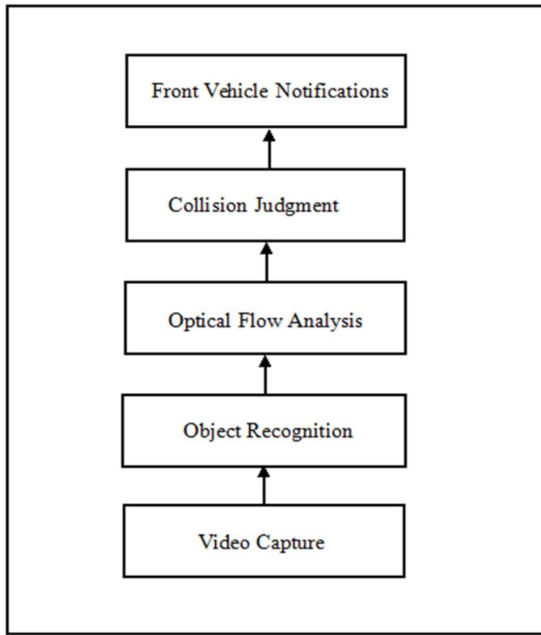
FIGURE 1. The flowchart of the proposed vehicle collision warning system
