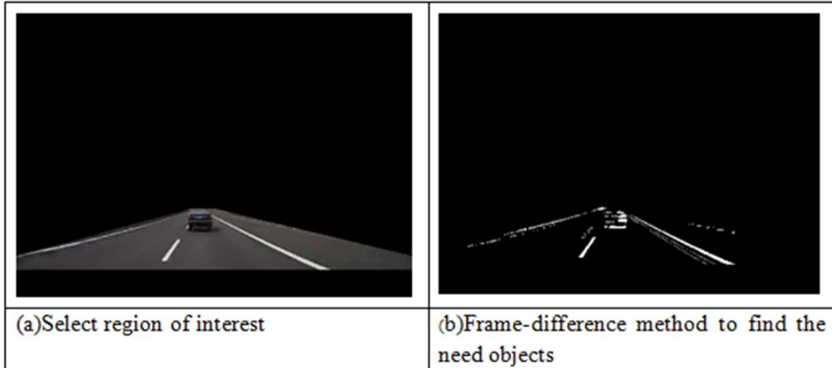
FIGURE 3. The simulation result of the difference frame method
