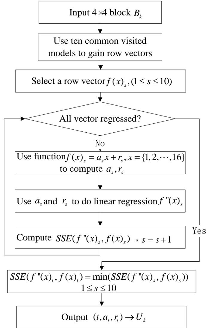
FIGURE 8. Flowchart using the linear regression coding method to compress a block  $B_k$  of an image
