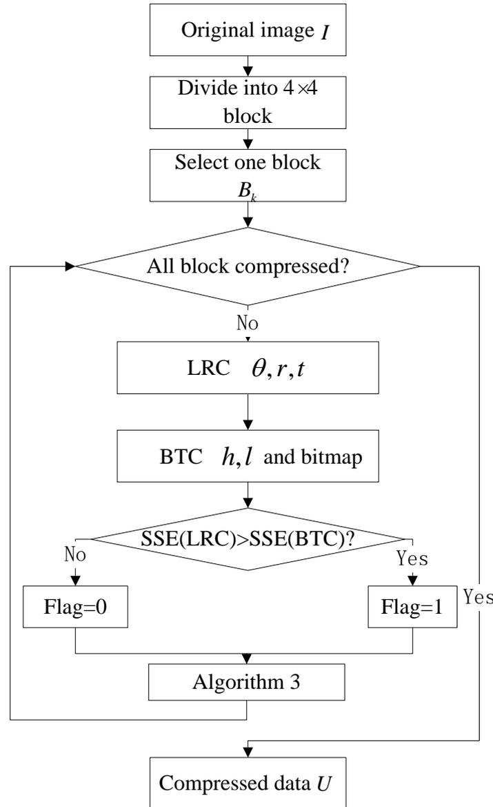
FIGURE 12. Flowchart of the proposed image compression method based on the BTC and LRC hybrid strategy
