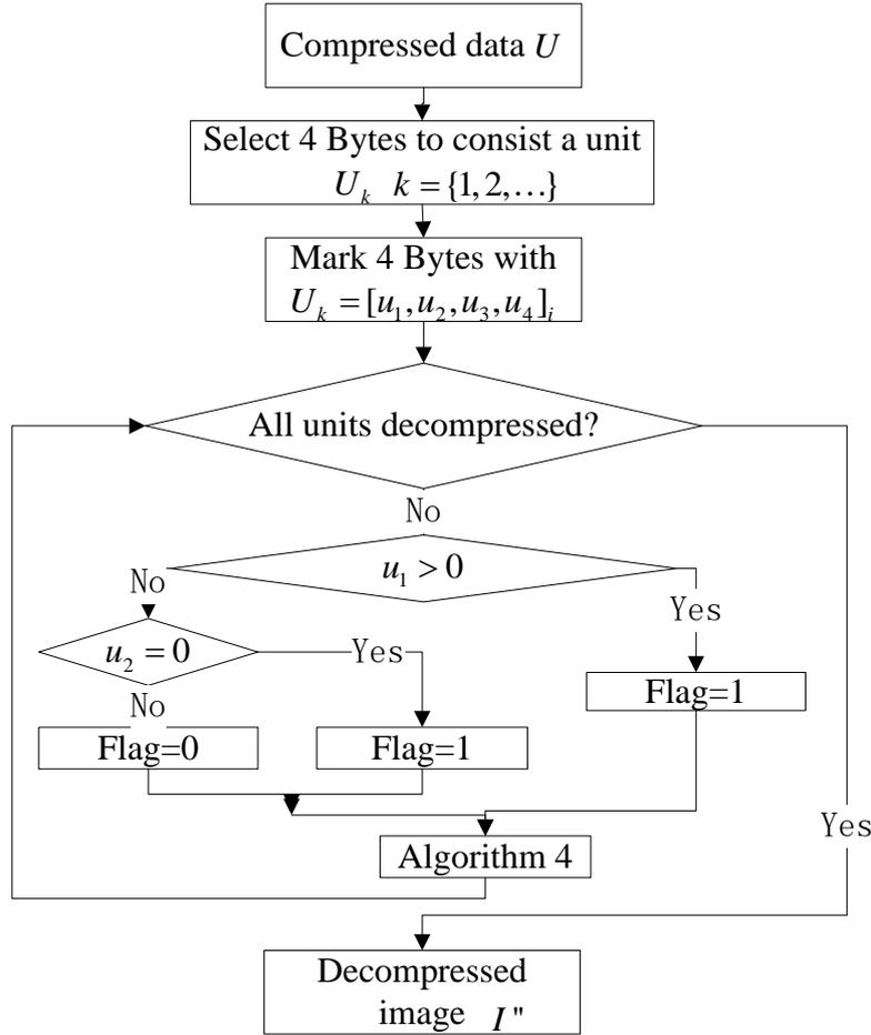
FIGURE 13. Decompression procedure of image compression method based on BTC and LRC hybrid strategy
