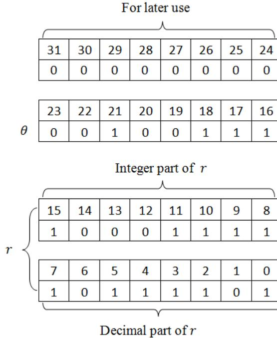
FIGURE 4. Organization of the 32-bit compressed unit with the LRC method
