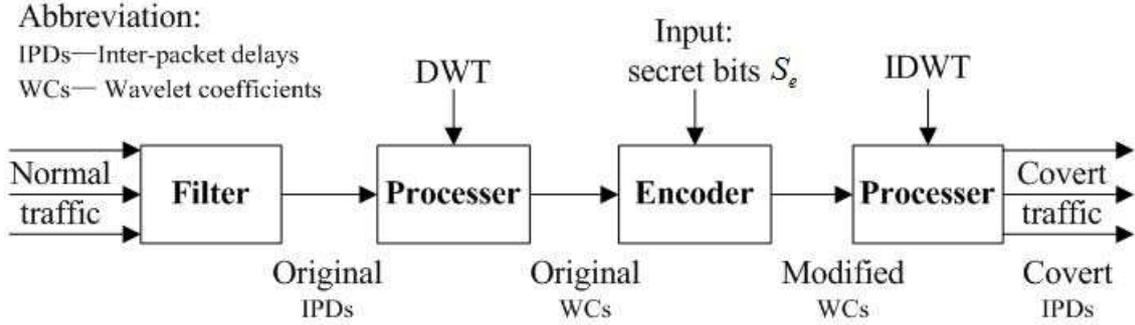
FIGURE 2. The model of our proposed covert channel
