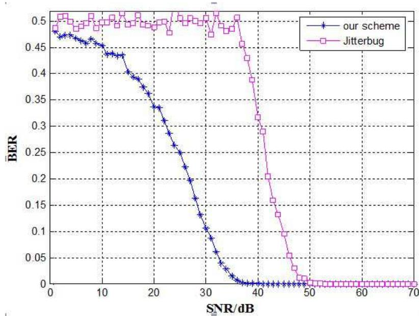
FIGURE 6. The comparison of BER between our scheme and Jitterbug under different SNR
