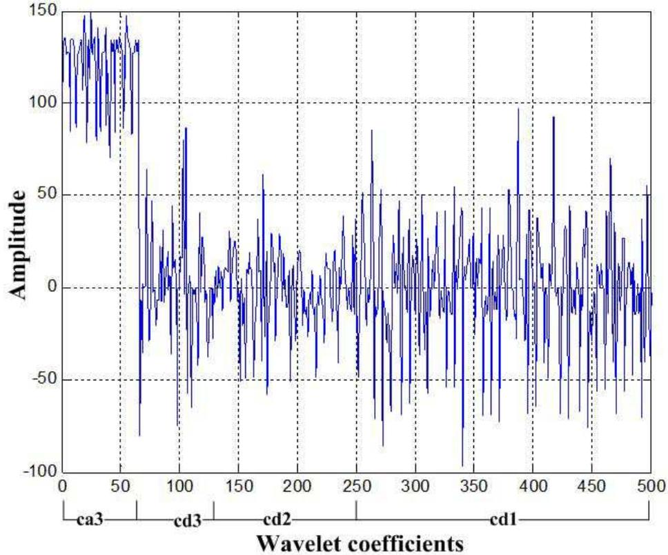
FIGURE 3. Three-level DWT of the original traffic
