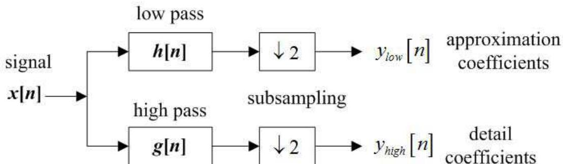
FIGURE 1. Wavelet decomposition of signal  $x$
