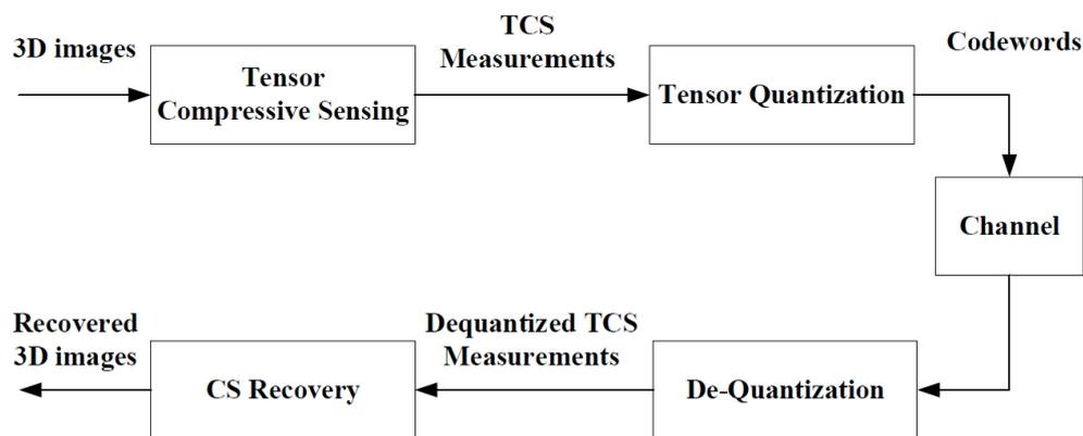
FIGURE 1. 3D CSI system framework designed via proposed method
