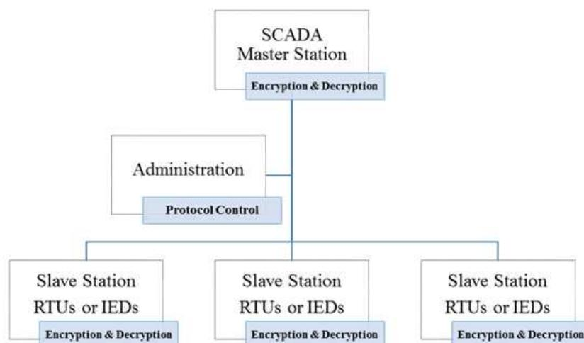
FIGURE 1. Typical SCADA network structure
