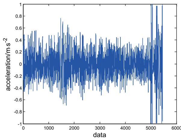
FIGURE 3. Time-domain waveform of gear box intermediate level acceleration
