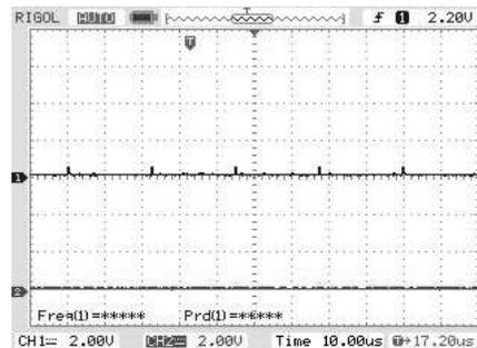
FIGURE 17. Burr signal after attenuation
