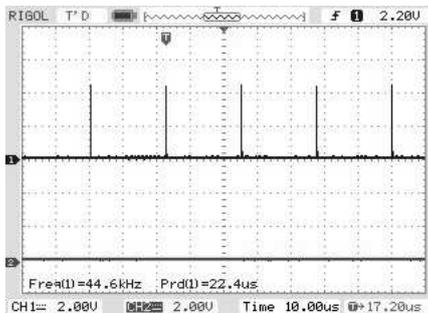
FIGURE 16. Signal interference burr
