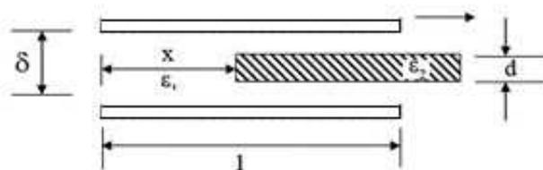
FIGURE 2. Variable dielectric constant capacitor
