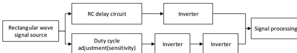
FIGURE 4. Rectangular wave generating circuit and F/V conversion circuit diagram
