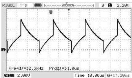
FIGURE 10. Capacitor charging and discharging waveform
