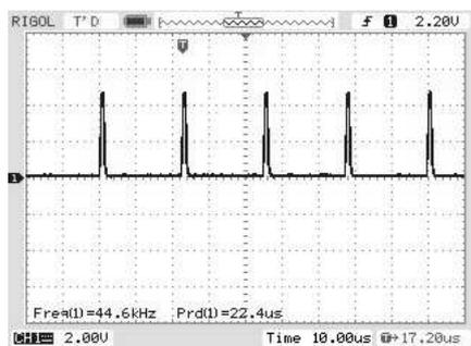
FIGURE 18. U1D invertin output spike
