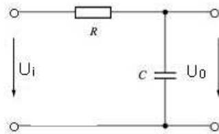
FIGURE 5. RC Delay circuit
