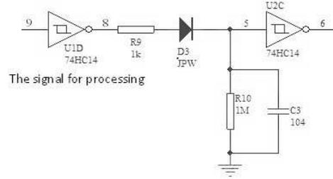
FIGURE 8. The signal for processing circuit
