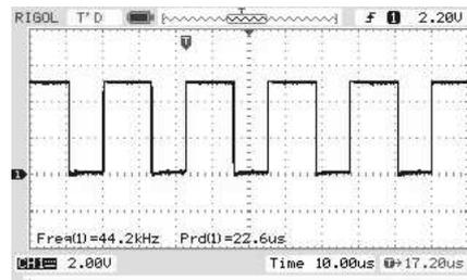
FIGURE 11. Multi harmonic oscillator output waveform
