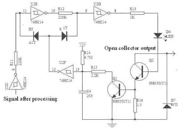
FIGURE 9. The output protection circuit
