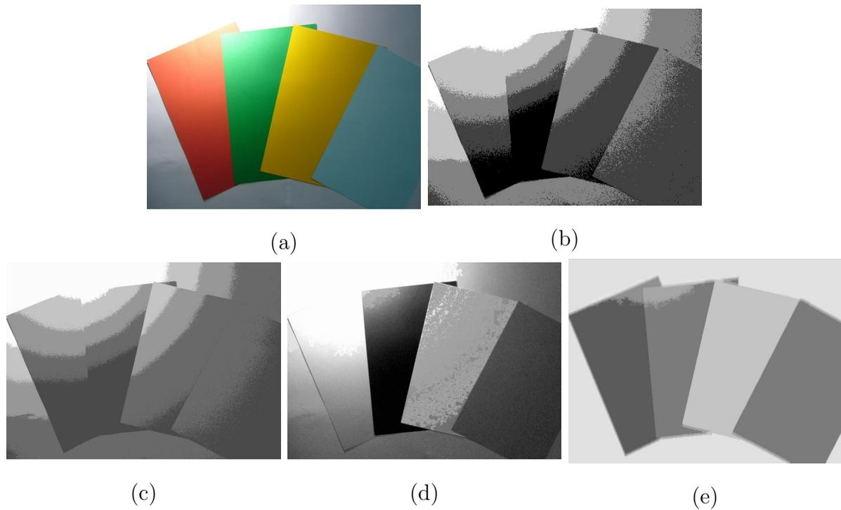
FIGURE 3. Segmentation Results on Papers Image: (a) Original image; (b) Segmentation Result based on Otu; (c) Segmentation Result based on K-Means; (d) Segmentation Result based on Mean-Shift; (f) Segmentation Result based on Color Constancy
