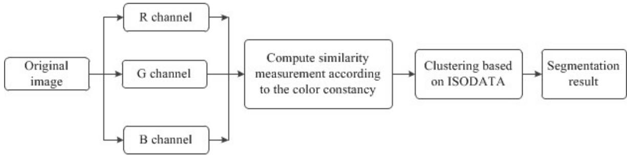
FIGURE 1. Processing Procedure of Segmentation Method Based on Color Constancy
