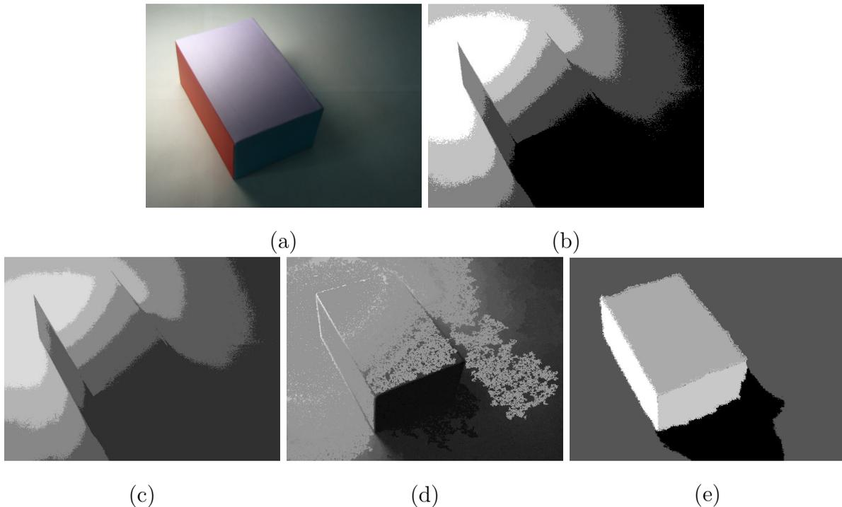
FIGURE 2. Segmentation Results on Cuboid Image: (a) Original image; (b) Segmentation Result based on Otsu; (c) Segmentation Result based on K-Means; (d) Segmentation Result based on Mean-Shift; (f) Segmentation Result based on Color Constancy
