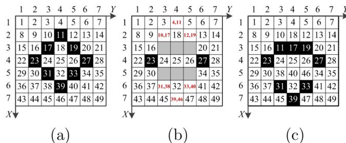
FIGURE 2. Proposed mesh warping (a) original image (b) preliminary warped image (c) final warped image
