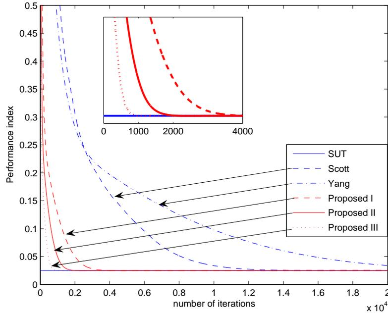
FIGURE 2. Average convergence curves with Gaussian signals
