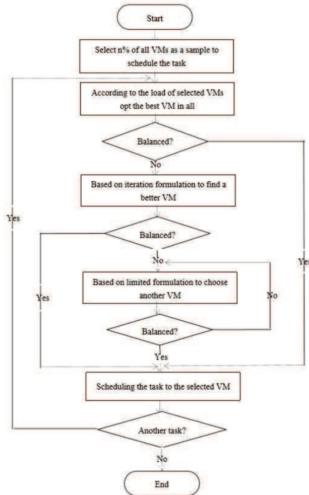
FIGURE 2. The proposed ABC algorithm based load balance method
