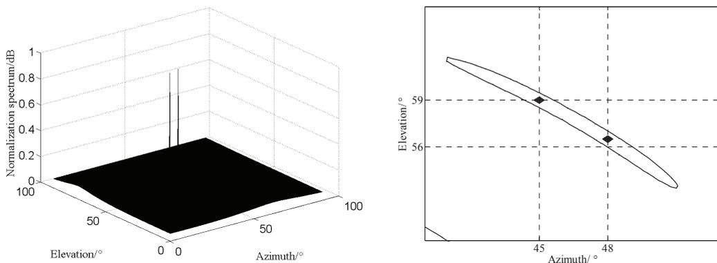
FIGURE 9. Normalization spectrum of TSRF for two near signals
