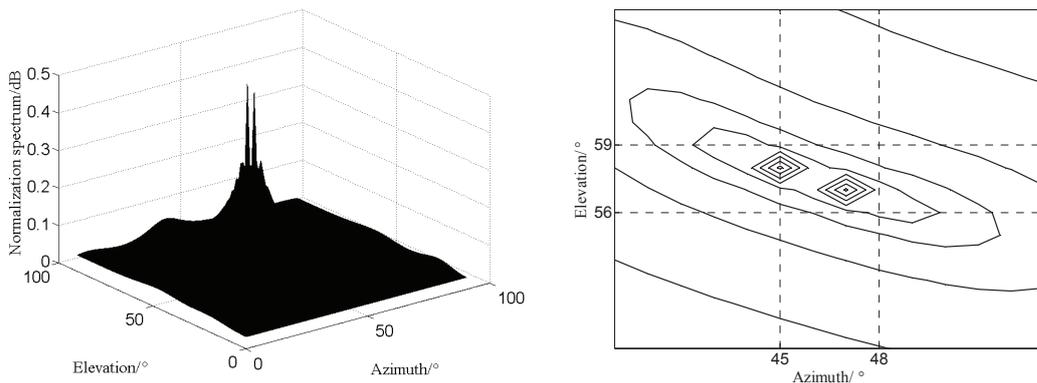
FIGURE 8. Normalization spectrum of SRD for two near signals
