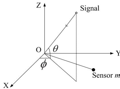
FIGURE 1. Array signal model
