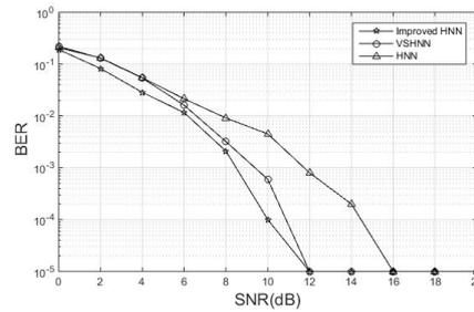
FIGURE 3. In one common zero channel, the error performance comparison of three algorithms.
