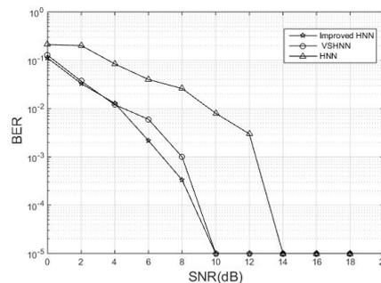
FIGURE 4. In Zhi Di channel, the error performance comparison of three algorithms.
