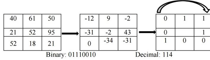
FIGURE 5. Example of  $3 \times 3$  LGP operator computation.
