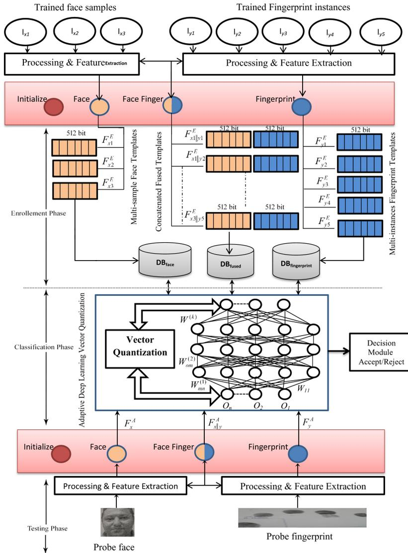
FIGURE 3. General schematic diagram for the proposed multimodal biometric system based on ADLVQ..
