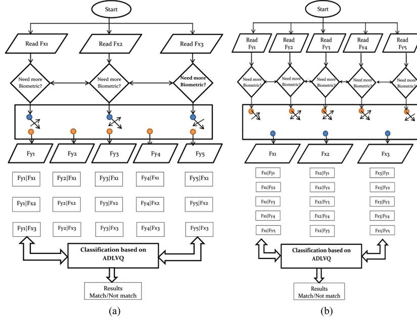
FIGURE 4. Testing phase of the proposed ADLVQ system with two scenarios: a) user enrolls face samples first. b) user enrolls fingerprint instances first.
