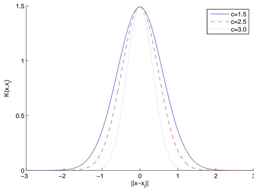
FIGURE 2. Kernel function curves with different  $c$  values
