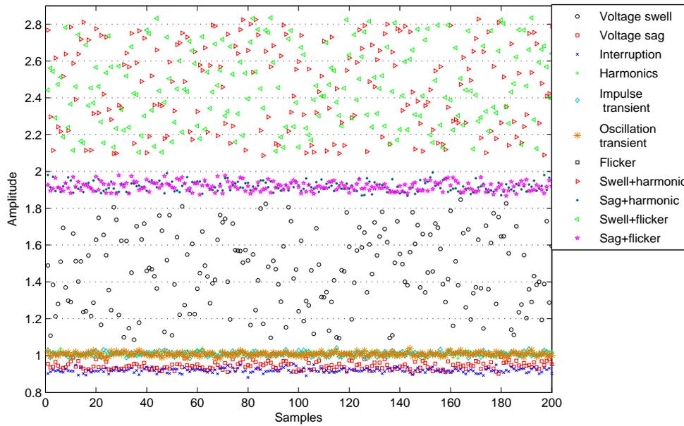
FIGURE 1. Relationship between the disturbance signals and their amplitudes for eleven kinds of disturbance
