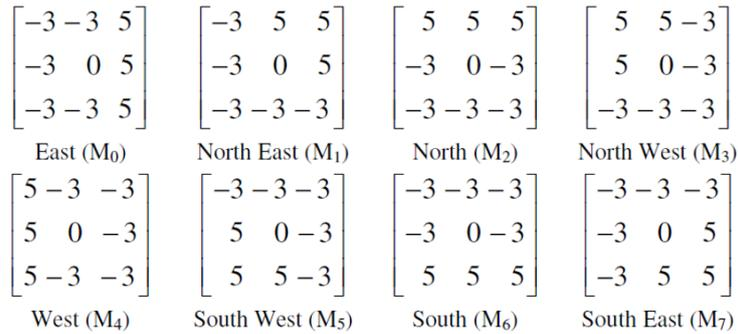
FIGURE 1. Kirsch edge response masks in eight directions.
