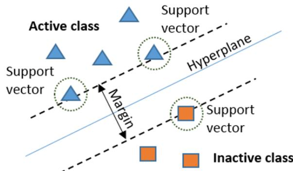
FIGURE 4. Maximum-margin hyperplane and margins for an SVM trained with samples from two classes.
