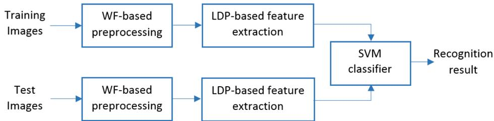
FIGURE 5. Block diagram of the proposed recognition system.
