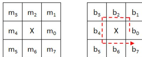
FIGURE 2. Edge response and LDP binary bit positions.
