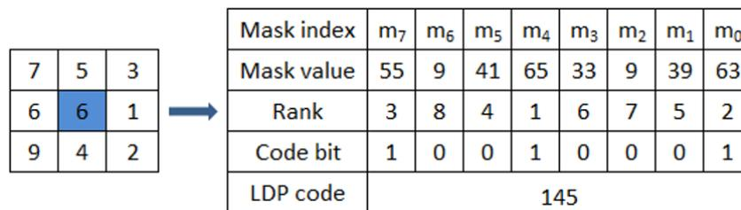
FIGURE 3. Generating LDP code with  $k=3$ .
