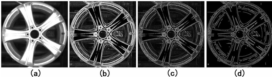
FIGURE 4. The steps of edge detection. (a)Original image. (b)Sobel transformation. (c)Non-maximal values suppression. (d)Hysteresis thresholding.
