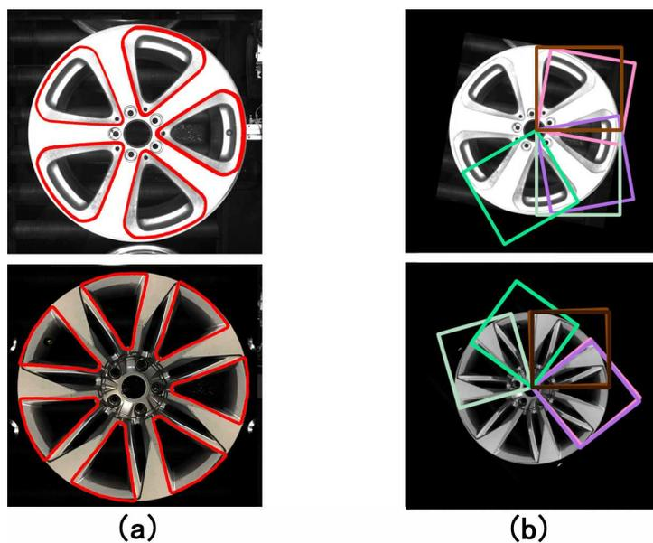
FIGURE 11. Comparing the results of two algorithm. (a)Results of proposed algorithm. (b)Results of pixel gray scale difference.
