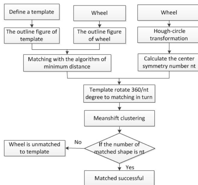
FIGURE 1. The process of wheel model recognition.
