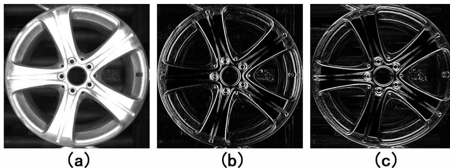
FIGURE 2. The effect of Sobel operator convoluted with original image. (a)Original image. (b)Transverse Sobel operator operation results. (c)Longitudinal Sobel operator operation results.
