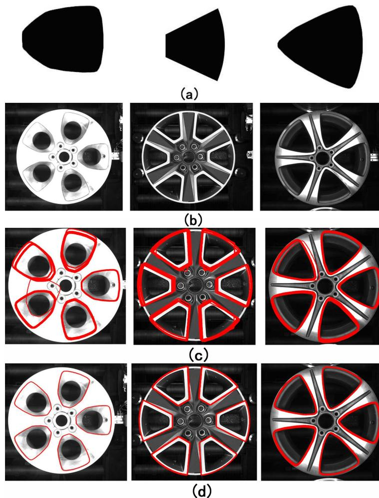
FIGURE 9. (a)Template of wheels A1-A3. (b)Wheel original images. (c)The matching results. (d)The result of the use of cluster meanshift.
