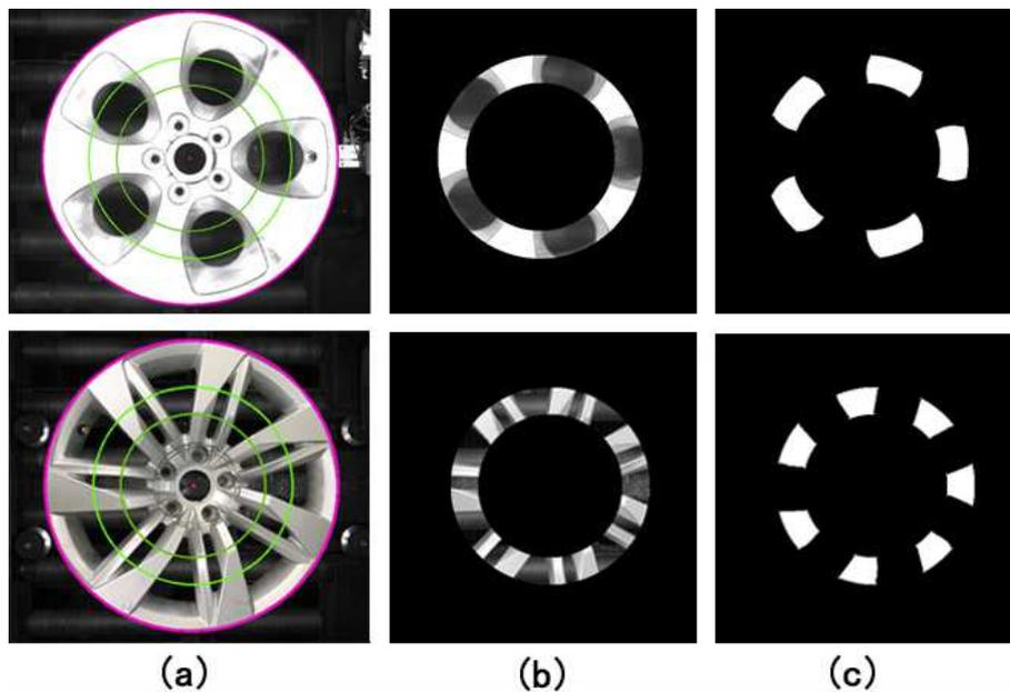
FIGURE 6. Calculating the center symmetry number. (a)Locating the extent of annular. (b)Extract annular region. (c)Binaryzation.
