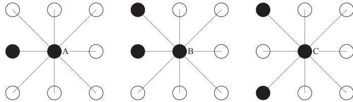
FIGURE 2. Example of edge endpoints
