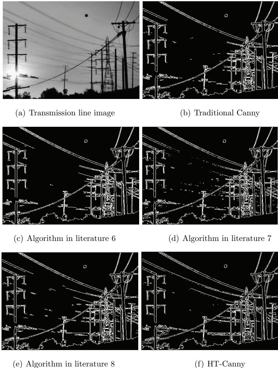
FIGURE 7. Edge detection results of Transmission Line image
