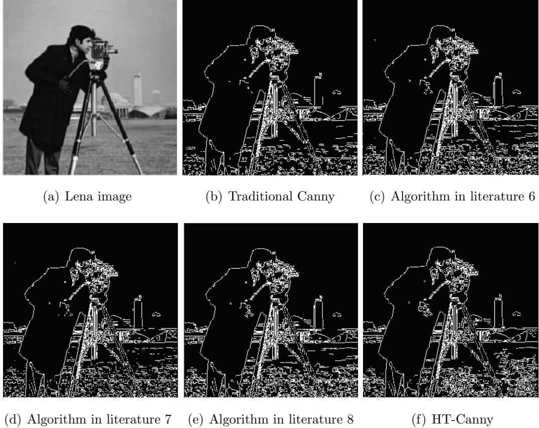
FIGURE 6. Edge detection results of Cameraman image
