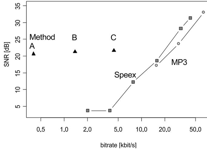
FIGURE 4. Quality of manipulated signal with respect to bitrate of the side information
