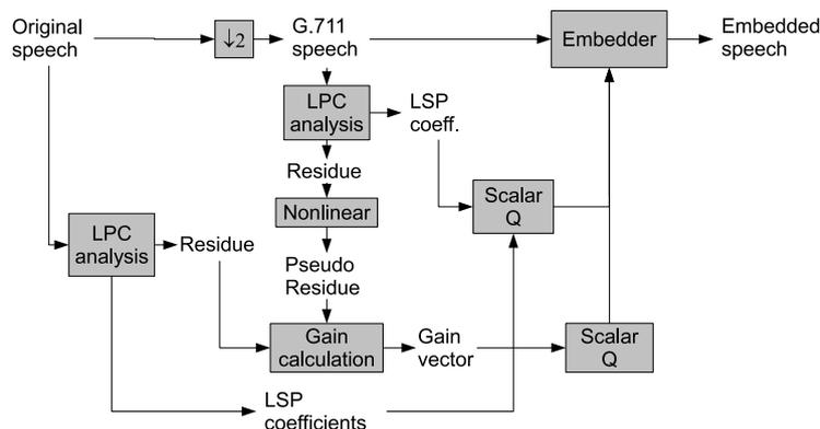
FIGURE 5. A block diagram of the encoder of telephone speech band extension
