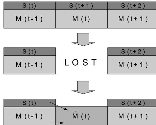
FIGURE 2. Packet loss concealment using sign information
