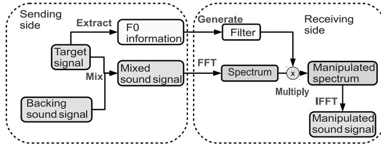
FIGURE 3. Signal manipulation using side information
