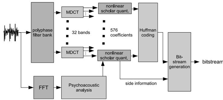
FIGURE 1. A schematic diagram of the MP3 encoder
