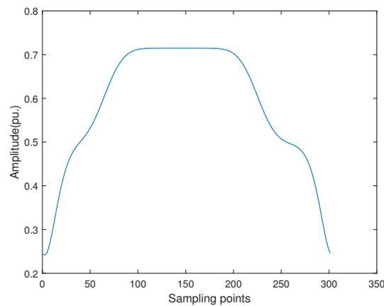
FIGURE 4. The Power Frequency Amplitude Curve Of improved S-transform
