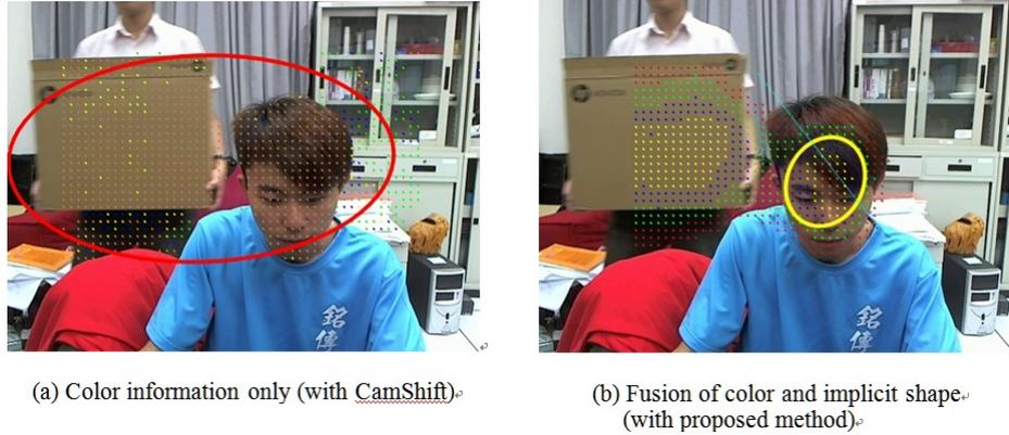
FIGURE 3. Probability distribution images generated in real case of tracking
