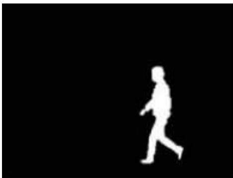
FIGURE 1. Sample of image silhouette extraction: Background subtraction image,
